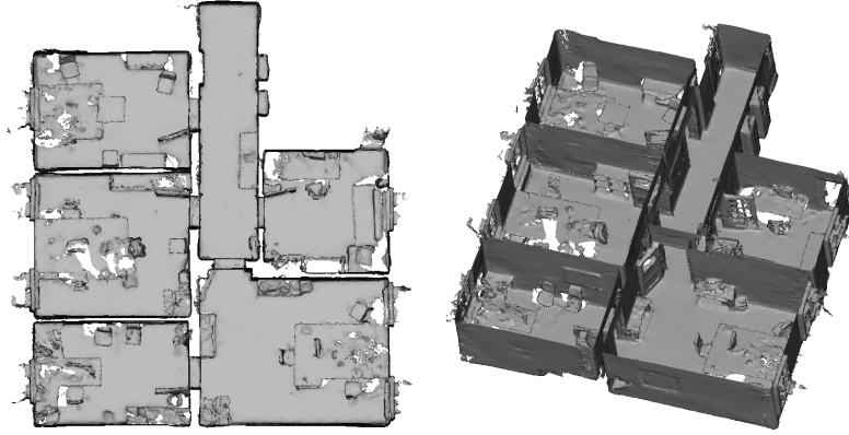
Figure 2.16: Triangle mesh of an indoor office environment captured by the HoloLens. The ceiling is removed for better visibility. Source: [238].
