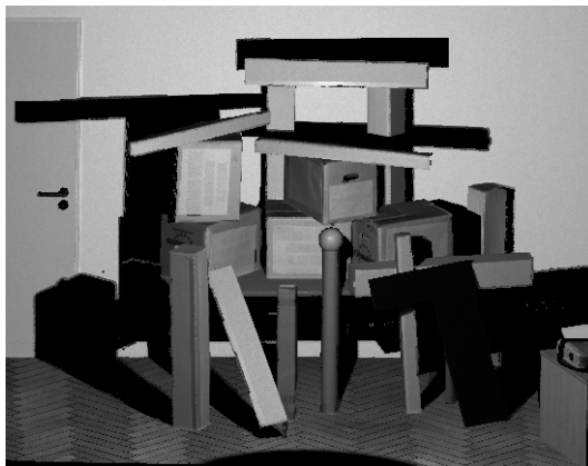
Figure 2.5: Ground truth data captured for a three-dimensional scene using a terrestrial laser scanner (Leica HDS6000). Source: [238].
