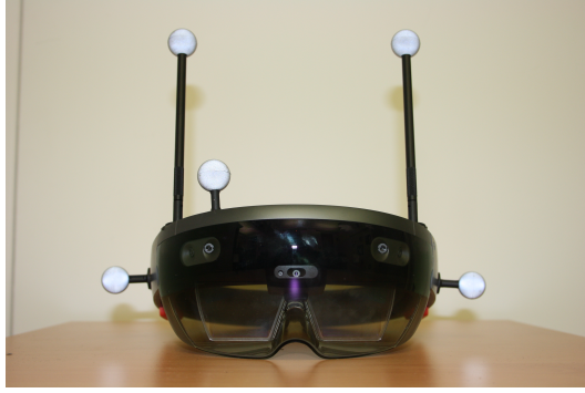
Figure 2.6: Rigid body of reflective sphere markers affixed to the HoloLens device. Source: [238].
