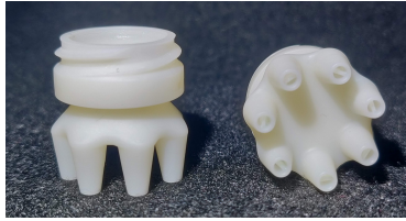
Figure 4.27: Side and bottom view of the circuitrode. The bottom view nicely displays the canals and cavities.
