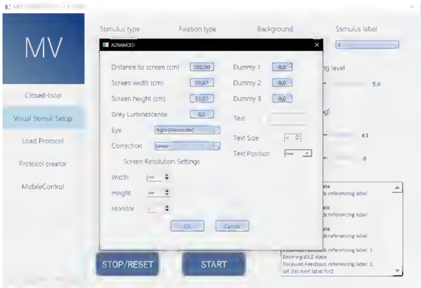
Figure 4.13: This screenshot shows the advanced settings which are possible to be set for the experiments. Important parameters are, for example, the distance of the subject to the screen, the screen size, the luminance, and rendering settings for VR. Furthermore, some dummy variables are available for the modification of complex or experimental stimuli.
