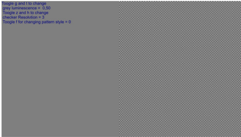
Figure 4.20: The screenshot shows the gamma calibration screen, which was implemented in unity. Half of the screen displays a grey value, the other half small black and white checkers. The screen is calibrated for luminance \gamma when the subject cannot perceive the difference between grey and checkerboard from the point of measurement.
