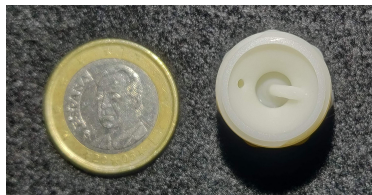
Figure 4.26: Top view of the circuitrode. A 1-Euro coin is displayed for scale. The entry-point for the syringe is on the left side of the electrode and the outlet for excess electrolyte is on the right.
