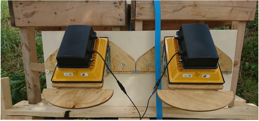
Figure 3.9: The used monitoring systems of the DeepBees study. When bees enter the hive through the entrance below the yellow boxes, they get recorded with the attached hardware. The hardware includes light sources and a camera.
