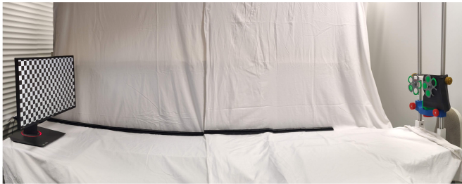
Figure 4.18: Side view on the Metis Videre laboratory setup. On the left, a high-frequency monitor is installed. On the right, the modular chin-rest is presented. The subject can sit on a chair which is provided. For reduced perceptual distraction, the rest of the optical table is covered in white linen.
