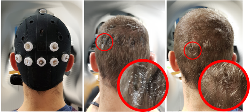
Figure 5.8: Comparison of state-of-the-art wet electrodes (center) and the circuittrodes (right). Both photos were taken directly after dismantling the EEG cap. The circuittrode leaves visibly fewer residues in the hair of the subject, making immediate showering obsolete.
