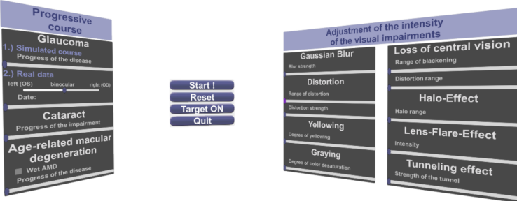
Figure 4.4: Display of the settings in the menu scene. On the right side, the strength of the different disease effects can be adjusted using sliders. On the left side, presets for progressive vision diseases can be selected. For glaucoma, it is possible to display imported perimetry data. A menu for basic functionality is provided in the center.
