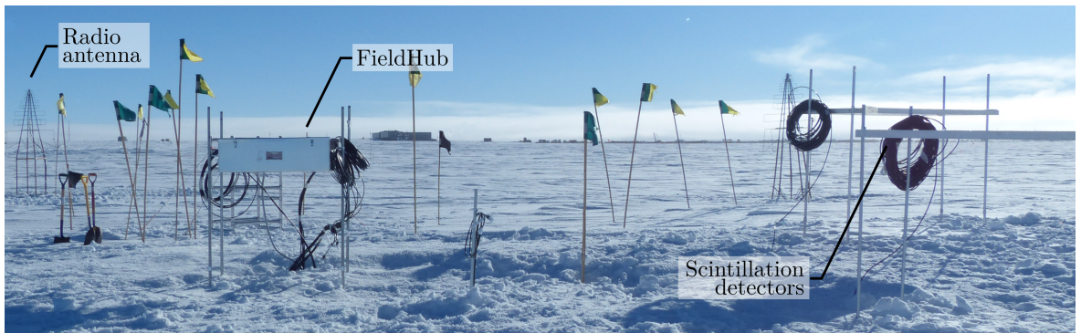
Figure 5.4: Photo of the center of the SAE prototype. The central DAQ is in the elevated FieldHub. The two central scintillation detectors (channel 0 and channel 1) can be seen on the right side. On the left side in the background, antenna A2 elevated on a new mount is visible. Picture credit: Marie Oehler, IceCube/NSF.
