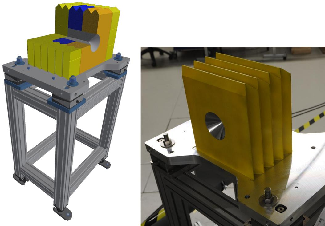
**Figure 2:** The electron beam dump. Left – CAD drawing, Right – realization of its core elements. The lead shielding can be added on demand. This option of a modular shielding extension is kept open if unexpectedly high beam currents (as, e.g., increased dark currents originating from the cathode and rf-cavity) have to be handled.
