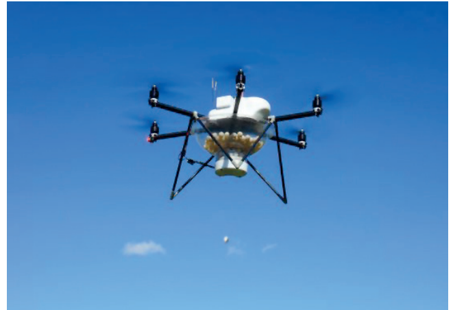
Fig. 2 Drone during the deployment of ichneumon wasps to fight corn borers
