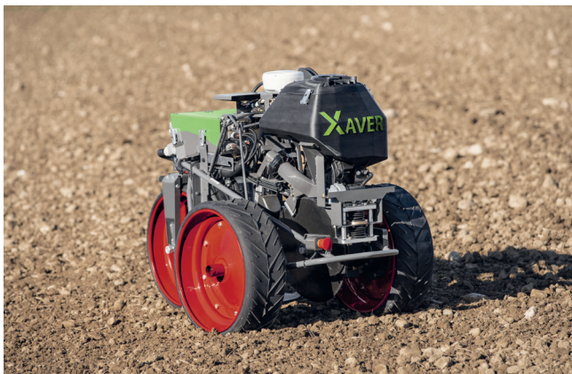
Fig. 3 »Xaver« by Fendt: robot units operating in a swarm
