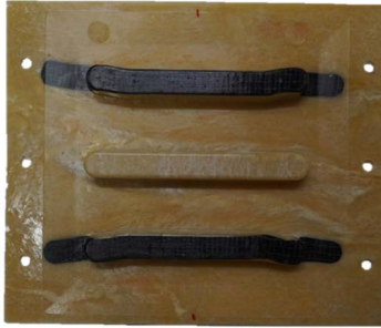
Figure 4.68: CoDiCo demonstrator part with optimized, I-shaped UD-tapes
