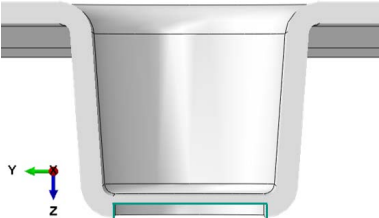
Figure 4.12: Example of a recess for a UD-tape in the part geometry used for the mold filling simulation in Moldflow
