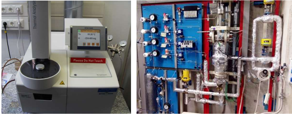
Figure 5: Thermogravimetric Analyzers. Left: Mettler Toledo TGA/ DSC 1 (Star System) Right: Non-commercial high-pressure TGA (up to 100 bar)
