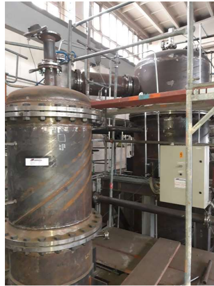
Figure 7: Fluidized bed gasification as part of the TC 2 -process - Thermo-Chemical-Conversion & Turbo-Compound-Concept (AG-Flue gas; BK-combustion chamber; BS-Fuel; G-Gear box and Generator; RG-Reaction gas; L-Air; M-Motor; RS-Residue; WS-Fluidized bed reactor; VD-Compressor; T-Turbine stages; Cyclone)
