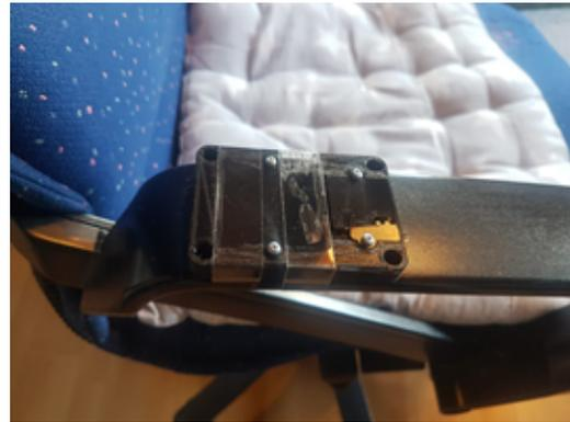
(b) Image of the encased sensor board attached to the armrest of the chair
