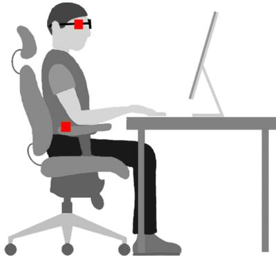
Figure 4.1: Sketch of the sensor placement (image taken from [42], modified). The red squares denote the position of the two sensors on the frame of wearable glasses and the armrest.
