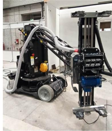
*Fig. 4: Manitou platform with shaver tool*
