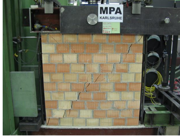
Figure 5.16: “WZI_0_2” specimen: damage state at the end of the first part of the test (DL3)
