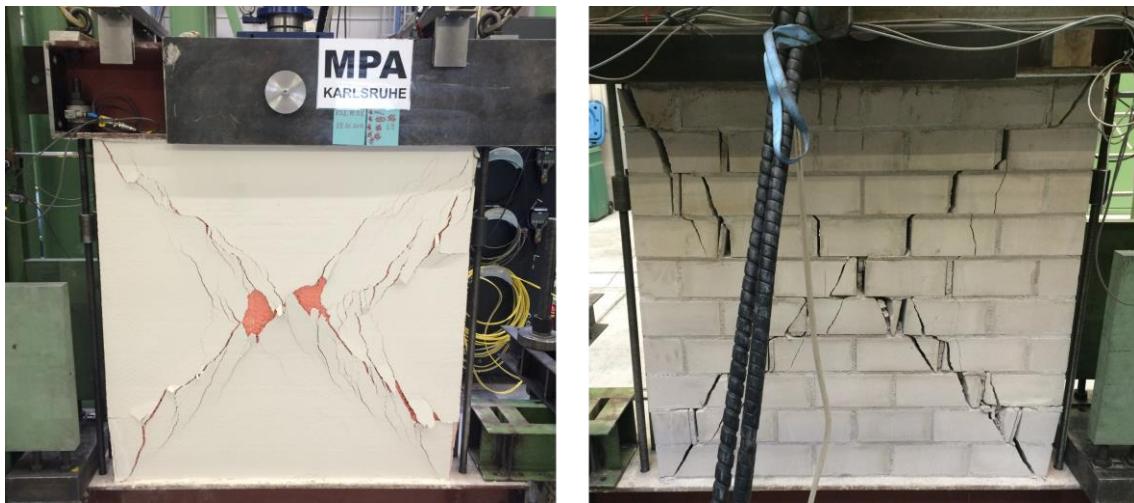
Figure 3.34: Final cracking pattern of the “KS_1_2” specimen
