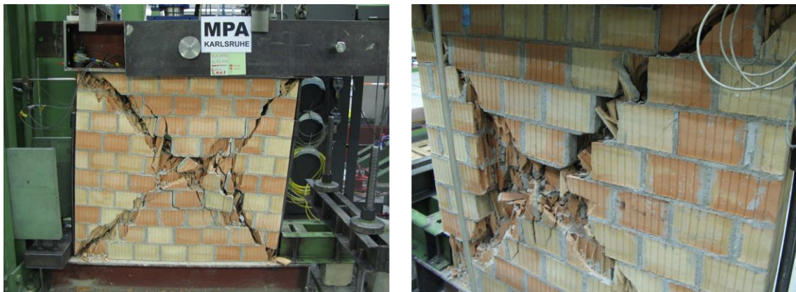
Figure 3.45: Final cracking pattern of the “WZI_0_2” specimen
