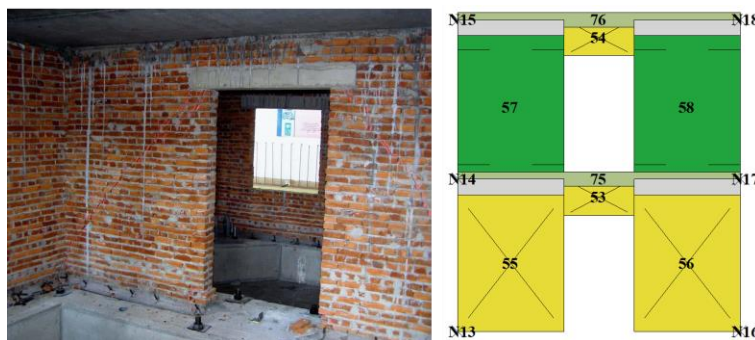
Figure 6.46: Experimental [73] and numerical final damage state of the P5 wall of the BM model (nonlinear dynamic analysis Petrovac 75)
