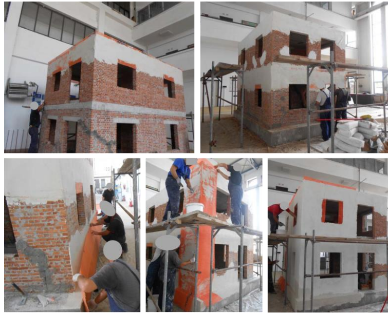
Figure 6.6: Retrofitting phases of the BM-SR model [73]
