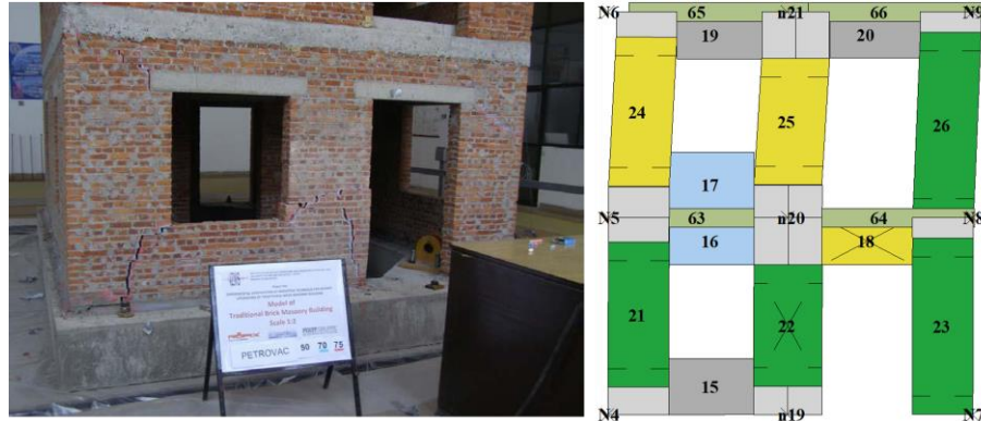
Figure 6.20: P2 wall of the BM model: experimental [73] and numerical final DLs (monotonic pushover in the +y direction with triangular inverse load pattern)
