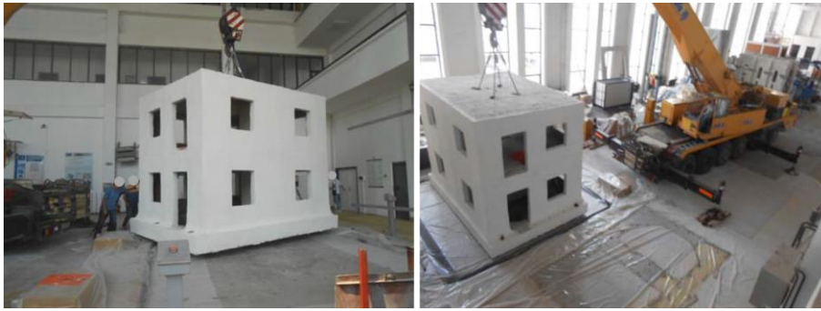
Figure 6.8: Transportation of the BM-SR model and positioning on the shaking table [73]
