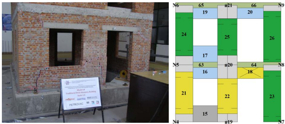
Figure 6.28: Experimental [73] and numerical final damage state of the P2 wall of the BM model (cyclic pushover with load pattern proportional to the masses)
