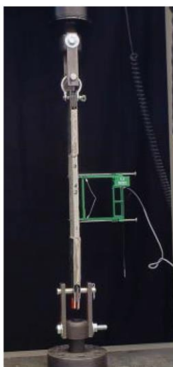
Figure 2.7: Uniaxial tensile tests with clevis-type grips on FRCM composite specimens [54]
