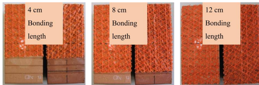
Figure 3.13: Double-lap shear-bond tests: bonding lengths
