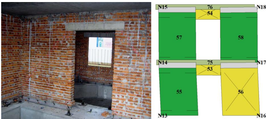
Figure 8.4: Wall P5 of the BM model: experimental [73] and numerical final DLs (monotonic pushover analysis in the -y direction with load pattern proportional to the masses)
