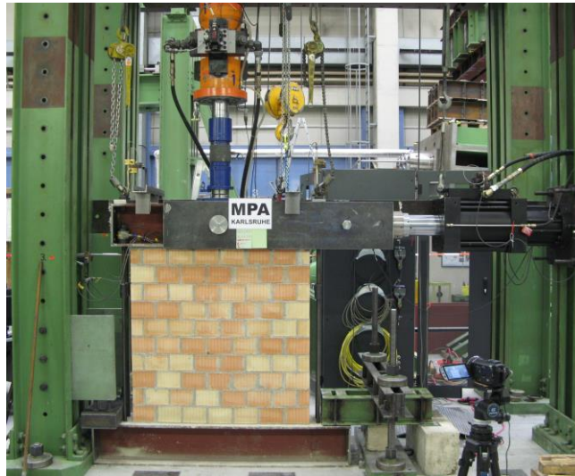
Figure 3.22: Cyclic lateral shear test: test setup
