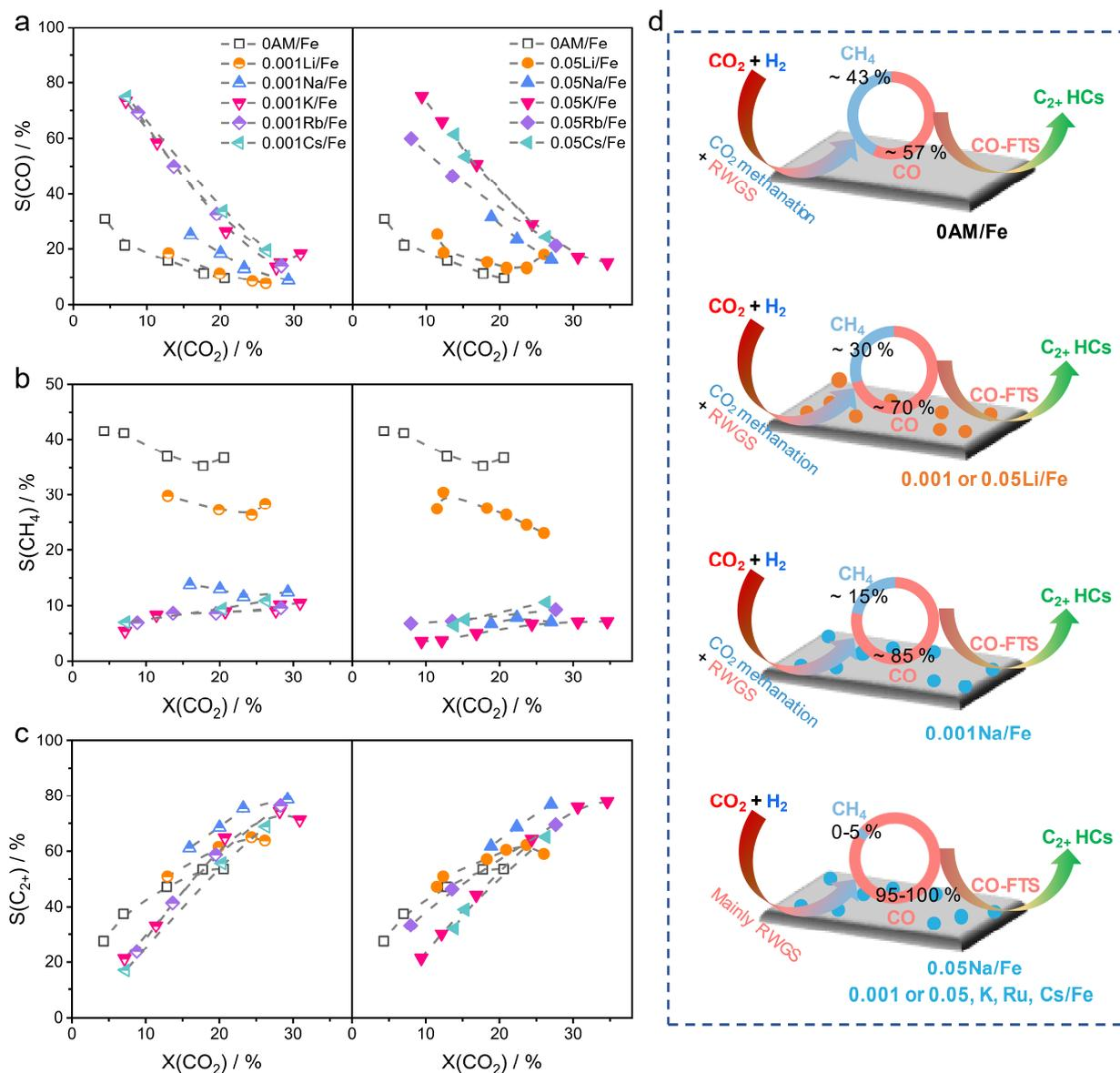
**Figure 4.** Selectivity-conversion relationships for (a) CO, (b) CH<sub>4</sub> and (c) C<sub>2+</sub>-hydrocarbons over 0AM/Fe and xAM/Fe catalysts. (d) Graphical representation of the reaction scheme of CO<sub>2</sub> conversion. The rings represent the product selectivity at zero CO<sub>2</sub> conversion. Reaction conditions: 300°C, 15 bar, H<sub>2</sub>/CO<sub>2</sub>/N<sub>2</sub> = 3/1/0.3, after 40 h on stream.
