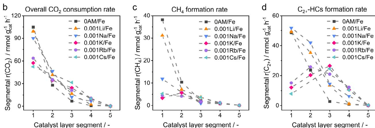
**Figure 3.** (a) Schematic representation how the segments (also see Scheme S1) are defined. The segmental rates of (b) overall  $\text{CO}_2$  consumption ( $r(\text{CO}_2)$ ), (c)  $\text{CH}_4$  formation ( $r(\text{CH}_4)$ ) and (d)  $\text{C}_{2+}$ -hydrocarbons formation ( $r(\text{C}_{2+})$ ) over OAM/Fe and 0.001AM/Fe catalysts. Reaction conditions:  $\text{H}_2/\text{CO}_2/\text{N}_2 = 3/1/0.3$ , 15 bar and  $300^\circ\text{C}$ .
