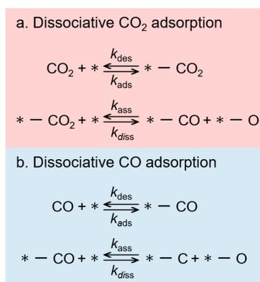
**Scheme 1.** Microkinetic models of reversible and dissociative adsorption of (a)  $\text{CO}_2$  and (b) CO.
