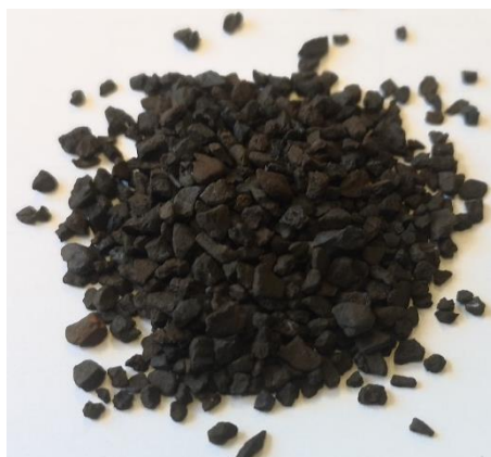
Figure 8.1: 1–3 mm big MnO 2 ore particles prior to synthesis.
