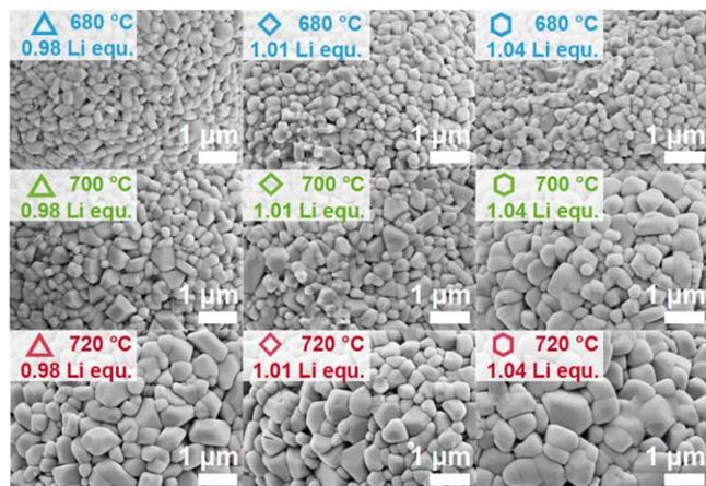
**Figure 2.** Top-view SEM images of the nominal 12  $\mu\text{m}$  LNO samples made with different Li equivalents and at different calcinations temperatures (see legends). All images were recorded in 20 k magnification with an acceleration voltage of 5 kV. A 6 nm thick Pt layer was sputtered onto all samples. The length of the white scale bar equals 1  $\mu\text{m}$ .
