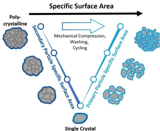
**Figure 11.** Schematic representation of the specific surface areas (SSAs) for different CAM morphologies. The left side represents the secondary, the right side the primary particle SSA that act as boundaries to the minimal/maximal accessible surface area of the CAM. By processes such as mechanical compression, washing and electrochemical cycling, the SSA increases by better accessibility of the inner pore structure. For single crystal materials, both boundaries converge to a single value.
