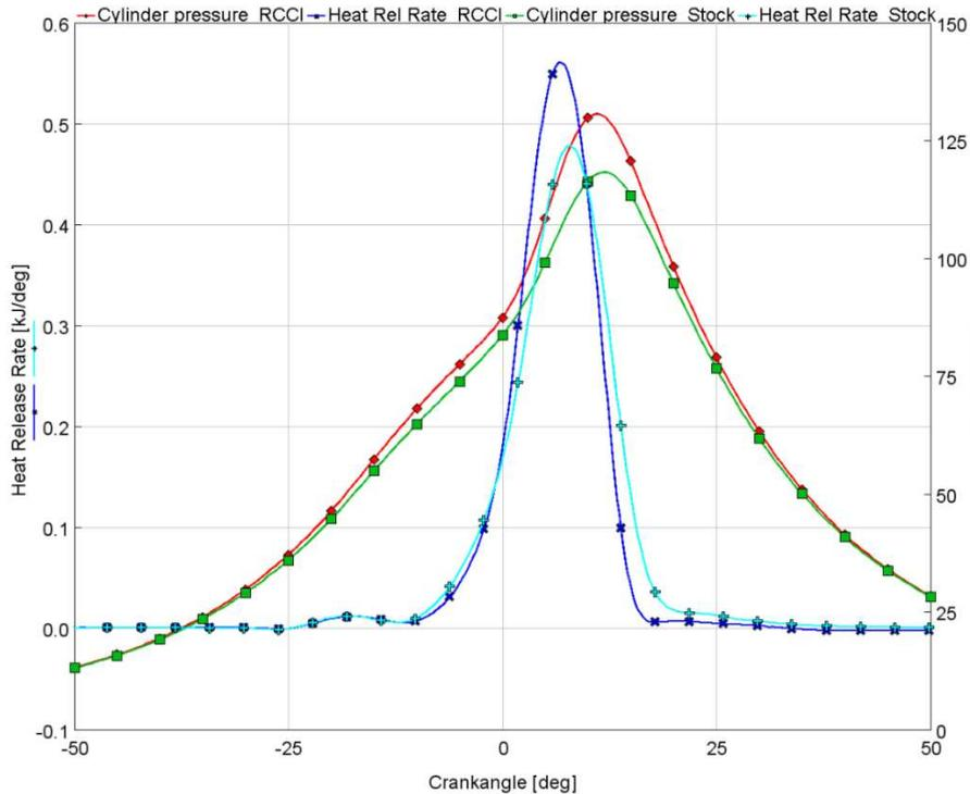
Fig. 9. Pressure and heat release trace over crankangle;  $\lambda=1.5$ ,  $P_2=2100\text{mbar}$ ,  $EGR=35$ ,  $CHI=0.83$ ,  $6300\text{J/Cycle}$ ,  $\epsilon=13.1$  stock and RCCI bowl with  $\epsilon=13.5$
