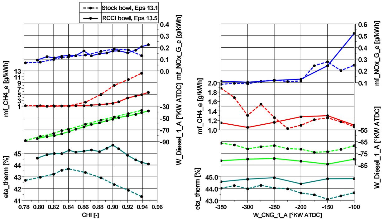
Fig. 8. CHI variation left, CNG SOI sweep right; Comparison of stock and RCCI bowl;  $\lambda=1.5$ ,  $P_2=2100\text{mbar}$ ,  $EGR=35\%$ ,  $6300\text{J/Cycle}$ ,  $\epsilon=13.1 / 13.5$
