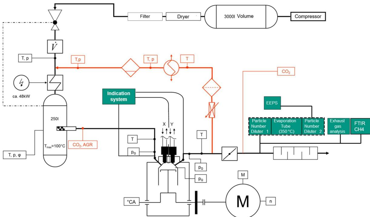
Fig. 3. Single Cylinder Testbench Scheme at KIT
