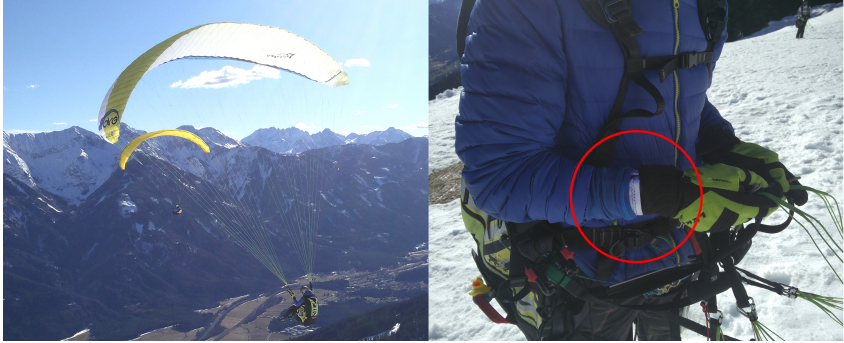
Figure 3.1: RüttelFlug is a wrist-worn tactile variometer, e.g. for paragliding. It was designed to be unobtrusive and fits well even under thick clothing.
