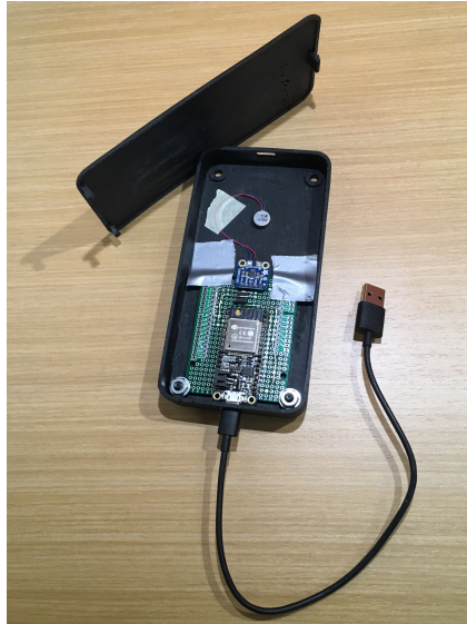
Figure 6.3: The dummy smartphone with the electronic components inside.
