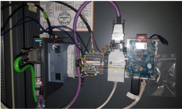
Figure 34 Use of the Smart Controller to integrate a Schaeffler SpindleSense sensor
