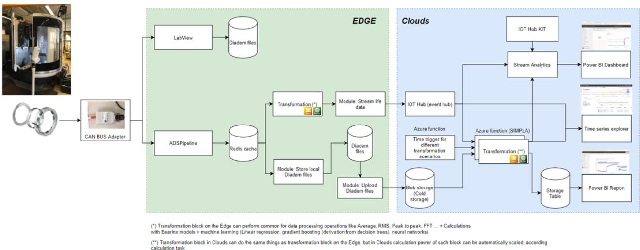
Figure 37 Solution Architecture – Schaeffler Azure Cloud
