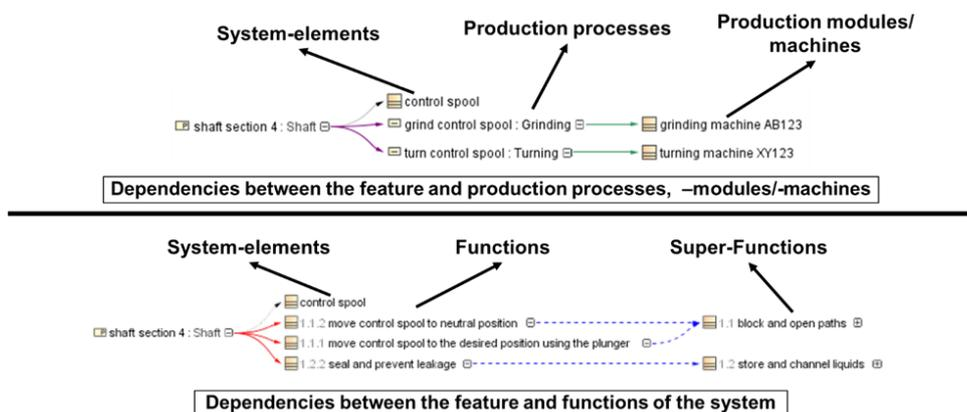
Figure 23 Analysis of the direct and implied dependencies from the feature shaft section 4
