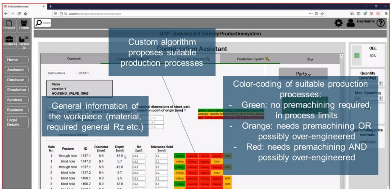
Figure 10 Proposition of suitable production processes based on the identified features
