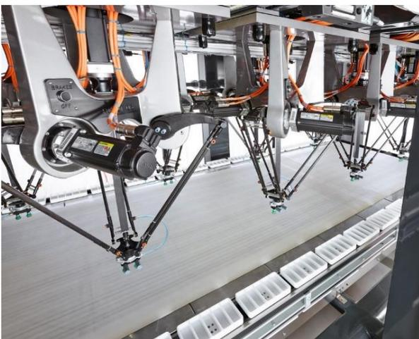
Figure 24 Delta robots
