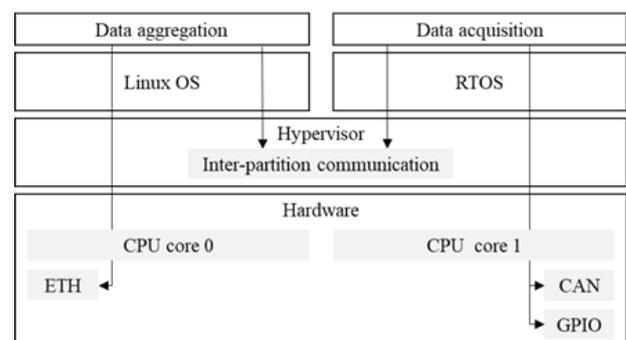
Figure 39 Smart Controller Architecture
