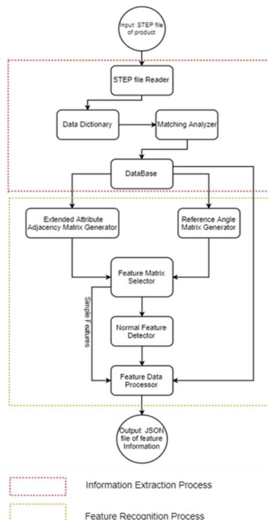
Figure 8 Custom algorithm for the Feature Extractor
