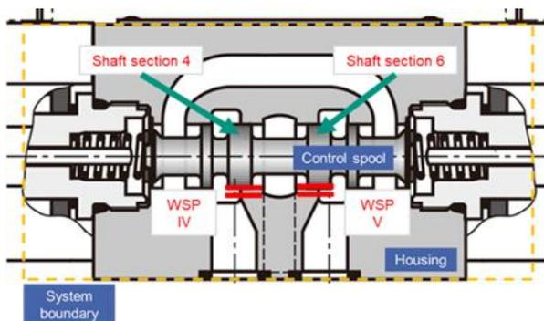
Figure 21 Section through the hydraulic valve, exemplarily displaying the parts “control spool” and “housing” as well as the features “shaft section 4/6” of the control spool
