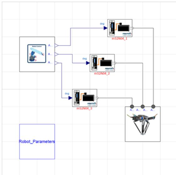
Figure 25 Simulation model of the delta robot
