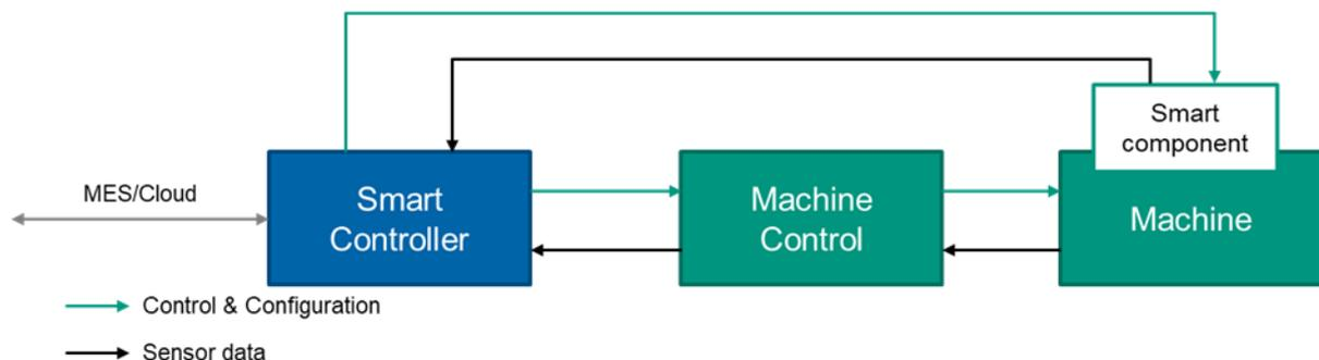
Figure 33 The „Smart Controller“ as a control unit for the acquisition of data from Smart Components and for communication with the machine control system.
