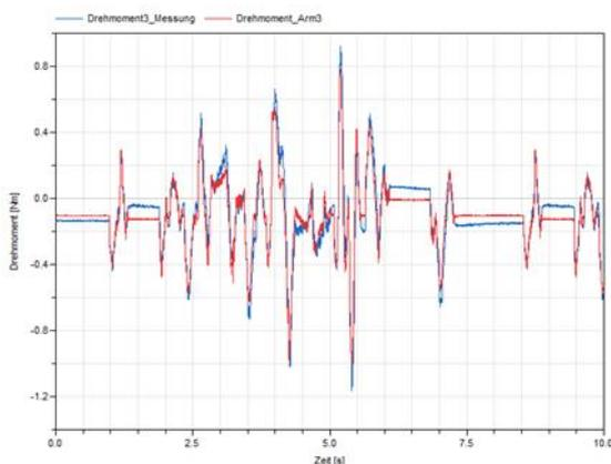
Figure 26 Measured and simulated torque
