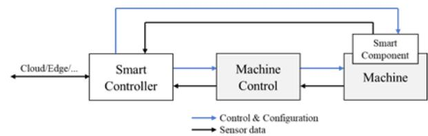
Figure 38 Smart Controller Interfaces
