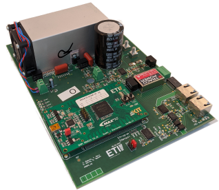
(c) A single SM of the MMSPC. The prototype has five SMs per phase.
