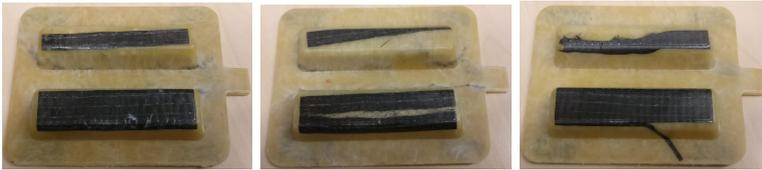
Figure 8.32: Patch defects observed in molded parts.
