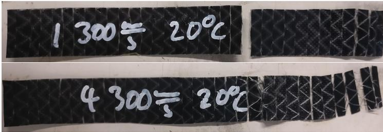
**Figure 7.11:** Tensile test with fibers oriented perpendicular to the loading direction are considered valid if failure occurs outside the clamped region. If progressive damage occurs in the clamped region, the test is considered invalid.
