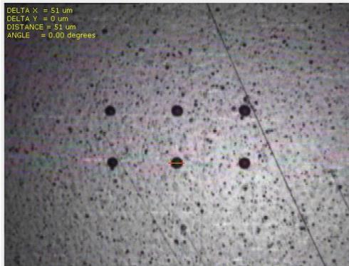
Figure 3.5: Printed droplets of silver ink. The droplet diameter was measured to be  $51\text{ }\mu\text{m}$ , therefore, the dot spacing was set to  $25\text{ }\mu\text{m}$ .
