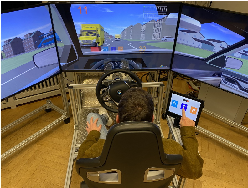
Figure 5.5: Front view of the driving simulator for highly automated driving equipped with three vehicle visualization screens (top), steering wheel and pedals (middle, unused in this experiment), a driver's seat (bottom) and a touchscreen as a maneuver decision interface (mid-right).
