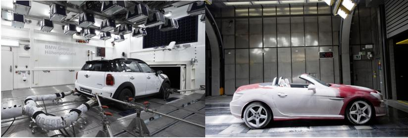
Figure 2.9: Examples of automotive manufacturer climate chambers [52,53]
