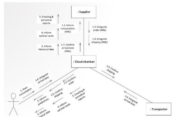
Figure 32: Communication Diagram Ekanban
