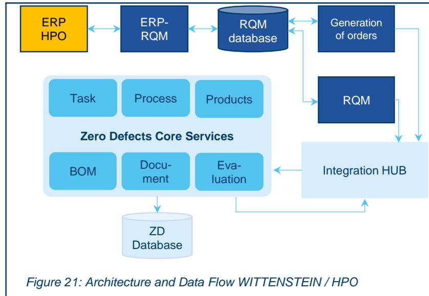
Figure 21: Architecture and Data Flow WITTENSTEIN / HPO
