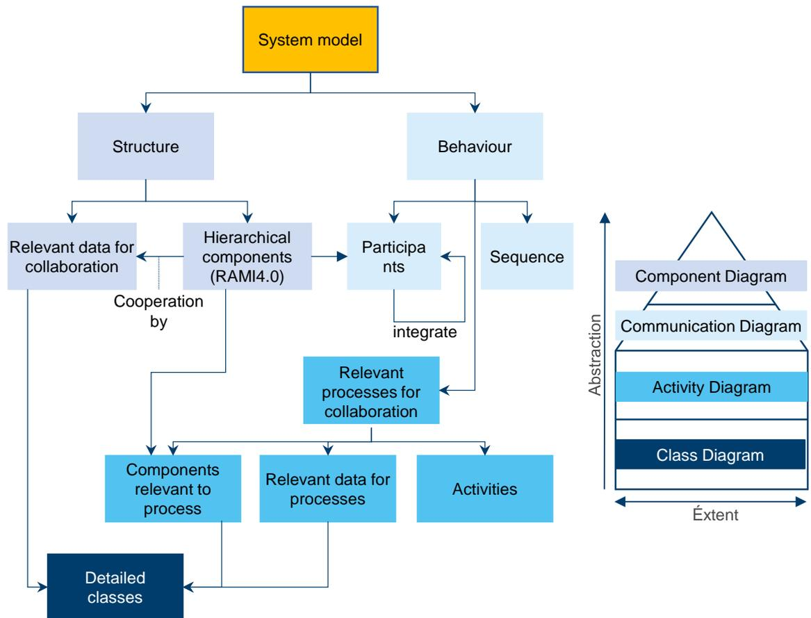
Figure 53: Representation of the Different Views of the System Model to Illustrate the Interaction Between the Different Diagrams (see. [26]).
