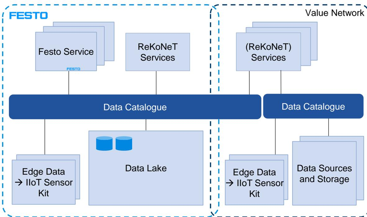
Figure 11: IT Architecture of the Recommender System
