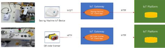
Figure 47: Vertical Sensor Integration into IOT Platform
