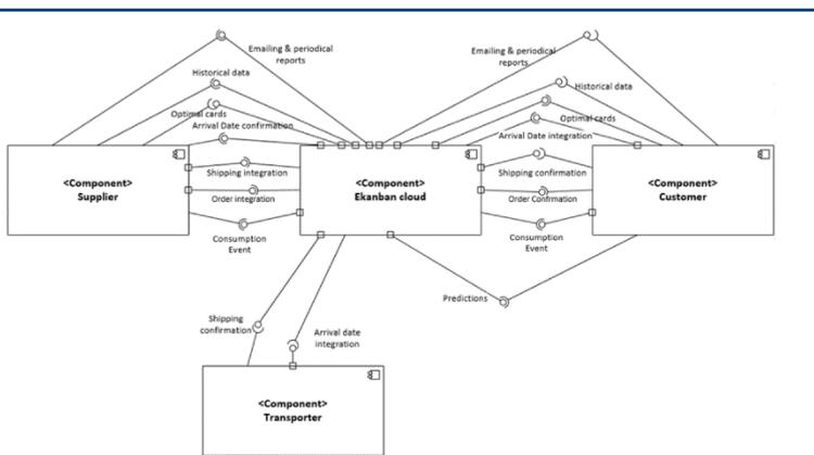
Figure 31: Component Diagram Ekanban
