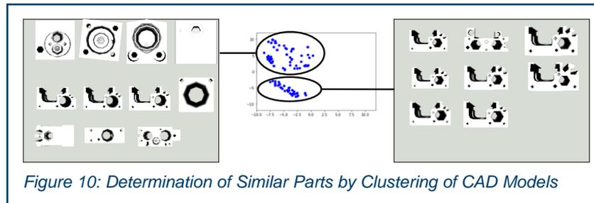
Figure 10: Determination of Similar Parts by Clustering of CAD Models
