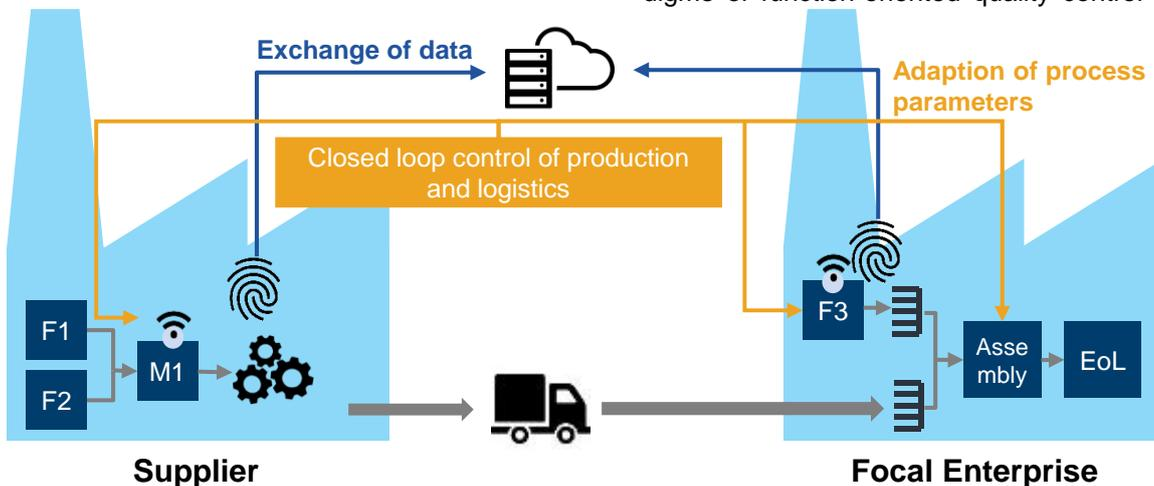
Figure 12: Target Vision of Cross-Company Quality Control ([15, 16])
