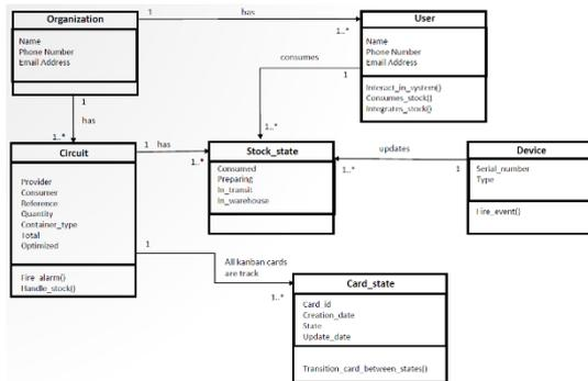
Figure 35: Class Diagram Ekanban
