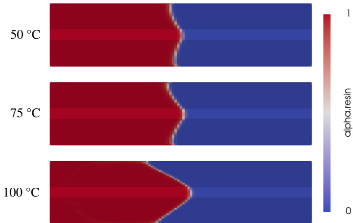
Figure 6.14: Flow front after 25 s for three temperatures with a foam core density of 100 \text{ g L}^{-1}
