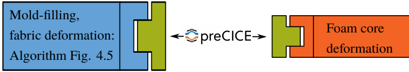
Figure 4.12: FSI coupling scheme to model sandwich manufacturing in RTM; the scheme consists of the internal coupling algorithm (Fig. 4.5) as the fluid part (blue) and the foam core solid mechanics (orange)
