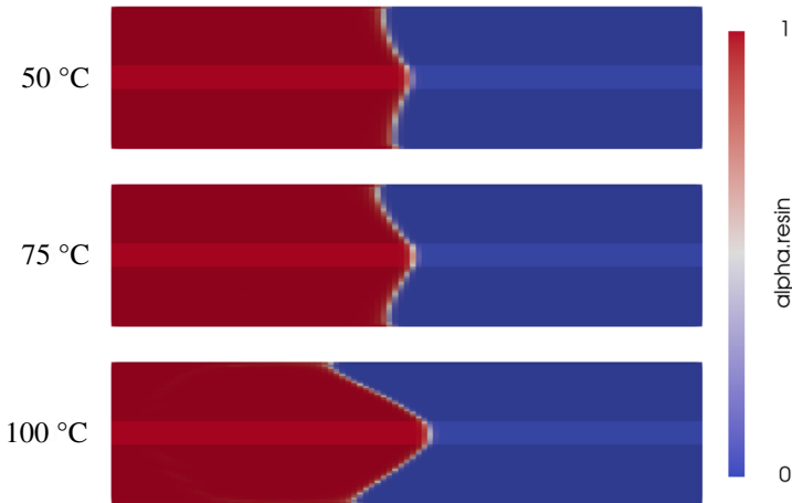
Figure 6.15: Flow front after 25 s for three temperatures with a foam core density of 130 \text{ g L}^{-1}
