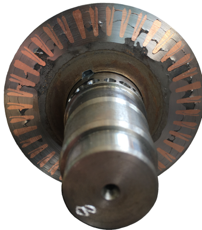
Figure 3.2: Electrical contact between steel and copper bars formed during production.
