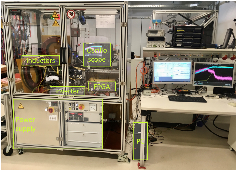
Figure 4.23: Test bench for double pulse method with installed inverter.
