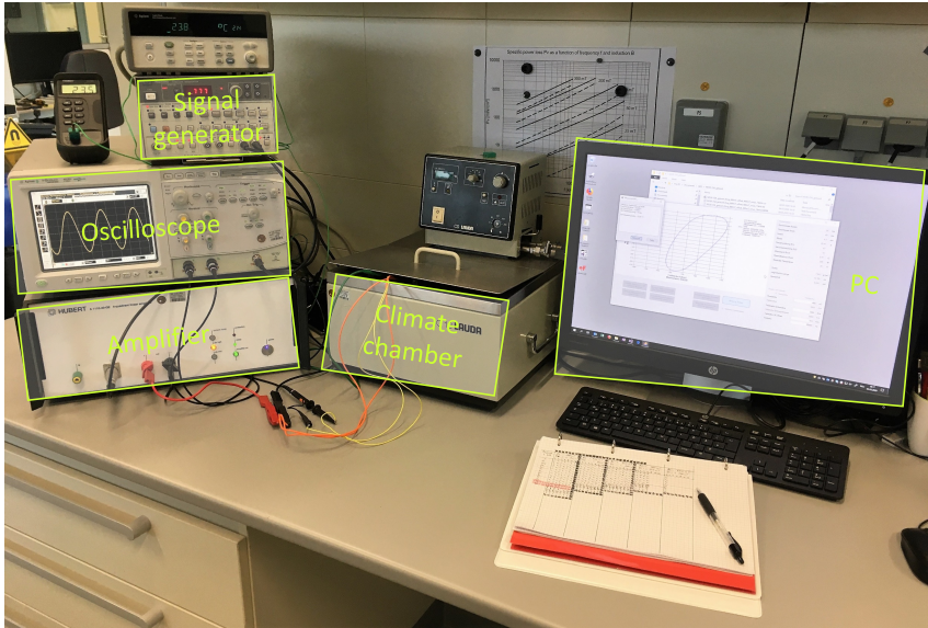
Figure 4.7: Test stand used for specific iron loss measurements.
