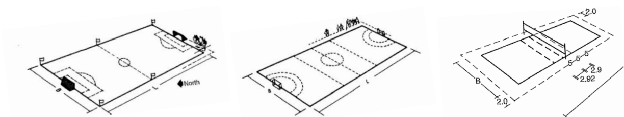
Figure 73 Orientation, dimensions and proportions of mini-football, handball and volleyball courts. Source: Neufert et.al, 2012
