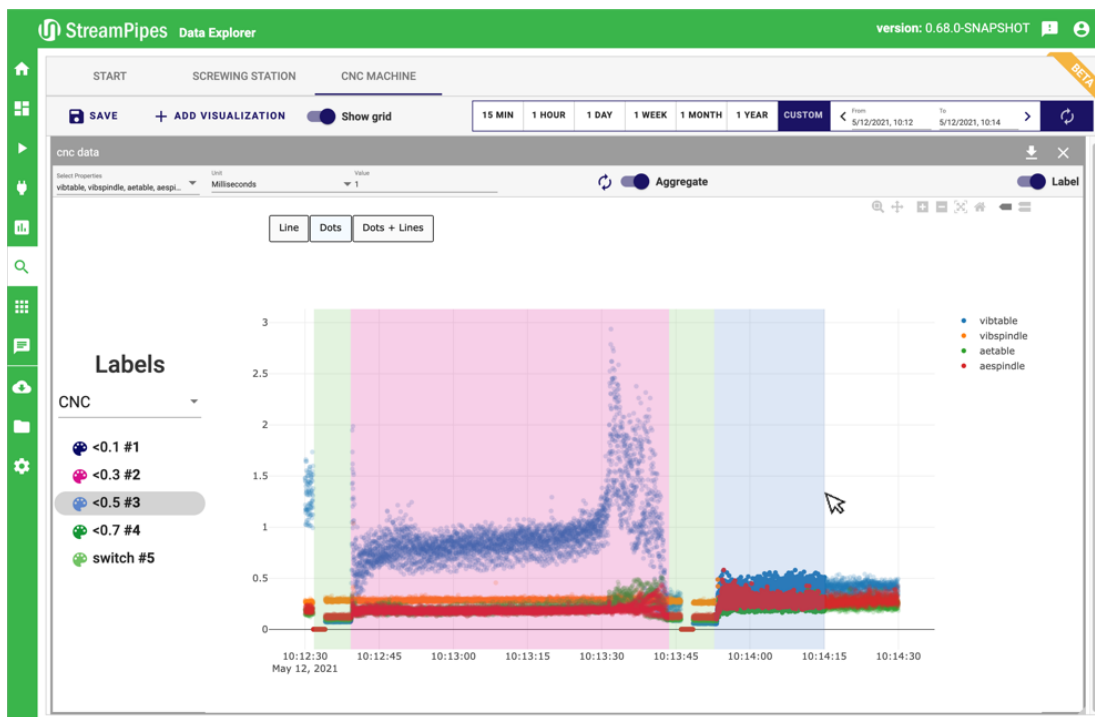
Figure 8.7.: Data explorer to visually analyze data and manually label event streams
