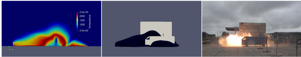
Fig. 12 – Temperature distribution (vertical slice crossing the jet nozzle), contour ( T = 1000 K) and the photo frame [21] after ignition ~ 80 ms
