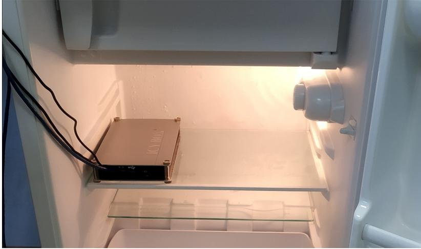
Figure 4.5.: Picture of one of the four boards encapsulated in a metal case inside an ordinary household refrigerator. Three cables coming out of the case are USB, Ethernet, and Power.
