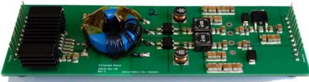
**Fig. 7:** Image of a single gate driver power supply unit.
