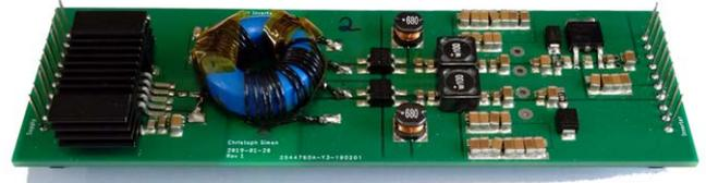
**Fig. 4:** Image of the gate driver power supply; each MOSFET has one, and it supplies galvanically isolated  $-4$  V to switch off and  $15$  V to switch on.
