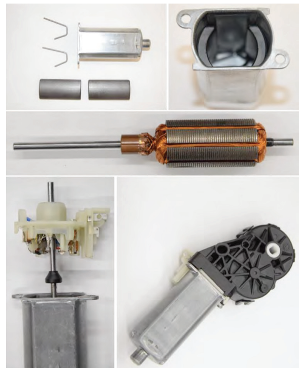
Figure 3: Bosch DC motor as demonstrator product of the learning factory
