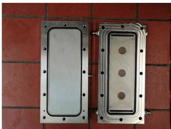
Flat sheet module. Feed side on the right and permeate side on the left.
