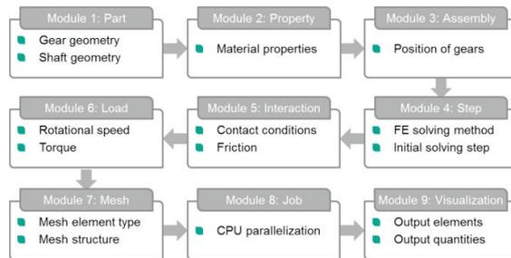
Fig. 3. Overview of the design of the FE model.
