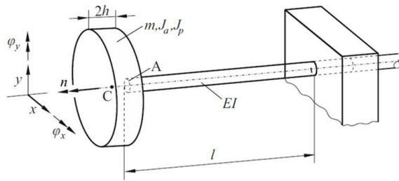
Fig. 6. Model of overhung rotor for the determination of the natural angular frequency of the shaft [14].
