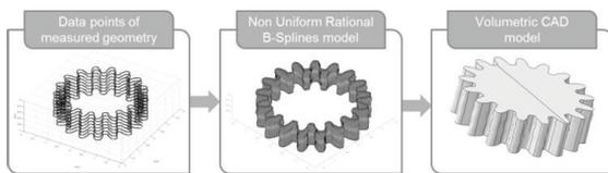
Fig. 4. CAD model of micro gears based on their measured geometry.
