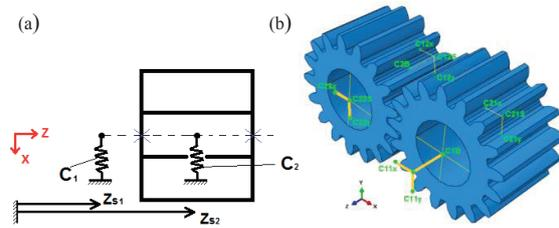
Fig. 5. (a) Euler Bernoulli model and (b) connector representation in Abaqus of the shaft geometry.
