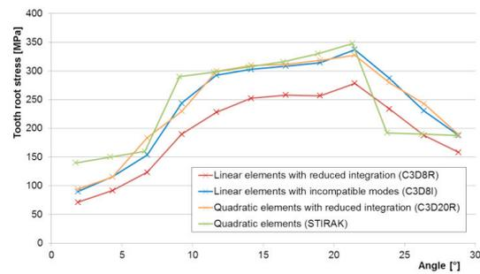
Fig. 7. Comparison of potential element types of the simulation model.
