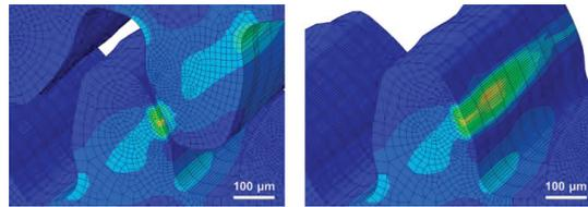
Fig. 2. FEM simulation of micro gears based on their measured geometry [6].
