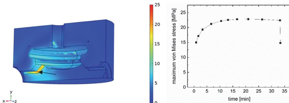
**Fig. 2.1.1:** Identification of critical thermally induced stress points (arrow, left) in the PP-housing of the KEA treatment chamber. Stationary values can be expected 17 minutes after start of operation, right.
