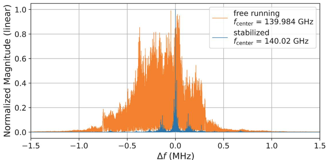
Fig. 1.8.1: Comparison of a free-running and PLL-stabilized gyrotron operation at W7-X.
