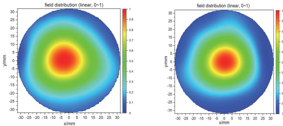
**Fig. 1.6.3:** Field distributions at the entry of the HE<sub>11</sub> waveguide: 170 GHz (left) and 204 GHz (right).
