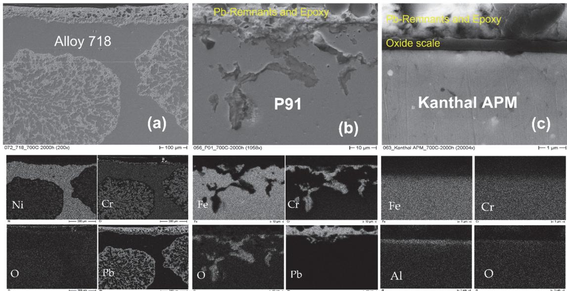
**Fig. 2.3.2:** Cross-sectional images and element distribution maps of (a) Alloy 718, (b) P91 and (c) Kanthal APM after 2000 h in stagnant Pb at 700 °C. Please note the different magnification in respective images.
