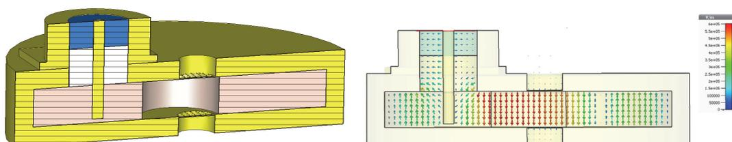
**Fig. 4.7.1:** (left) Cross-sectional view of the microwave applicator intended for virus inactivation using E-fields, and (right) its E-field profile.
