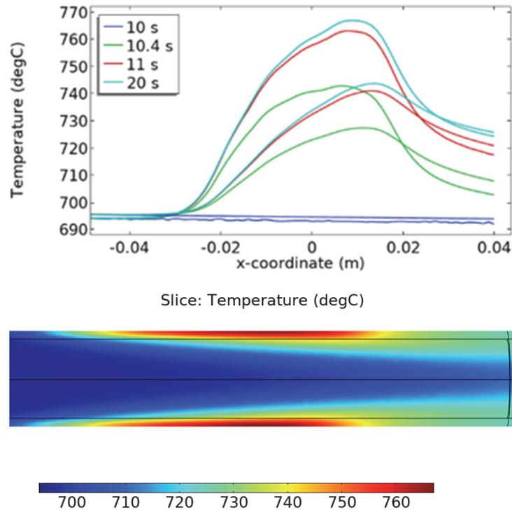
**Fig. 2.3.1:** Transient temperature distribution. Left column: Temperature profile along outer respectively inner side of lower wall of test tube at different time moments (inductive heating is switched on after 10 s). Right column: Stationary temperature distribution.
