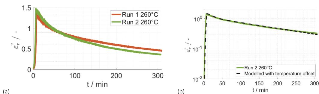
Fig. 4.3.2: First result of microwave heated PAN fiber. (a) Dielectric loss of the same process parameters measured at different runs. (b) Logarithmical comparison between measured dielectric loss and fitted values using a temperature offset.
