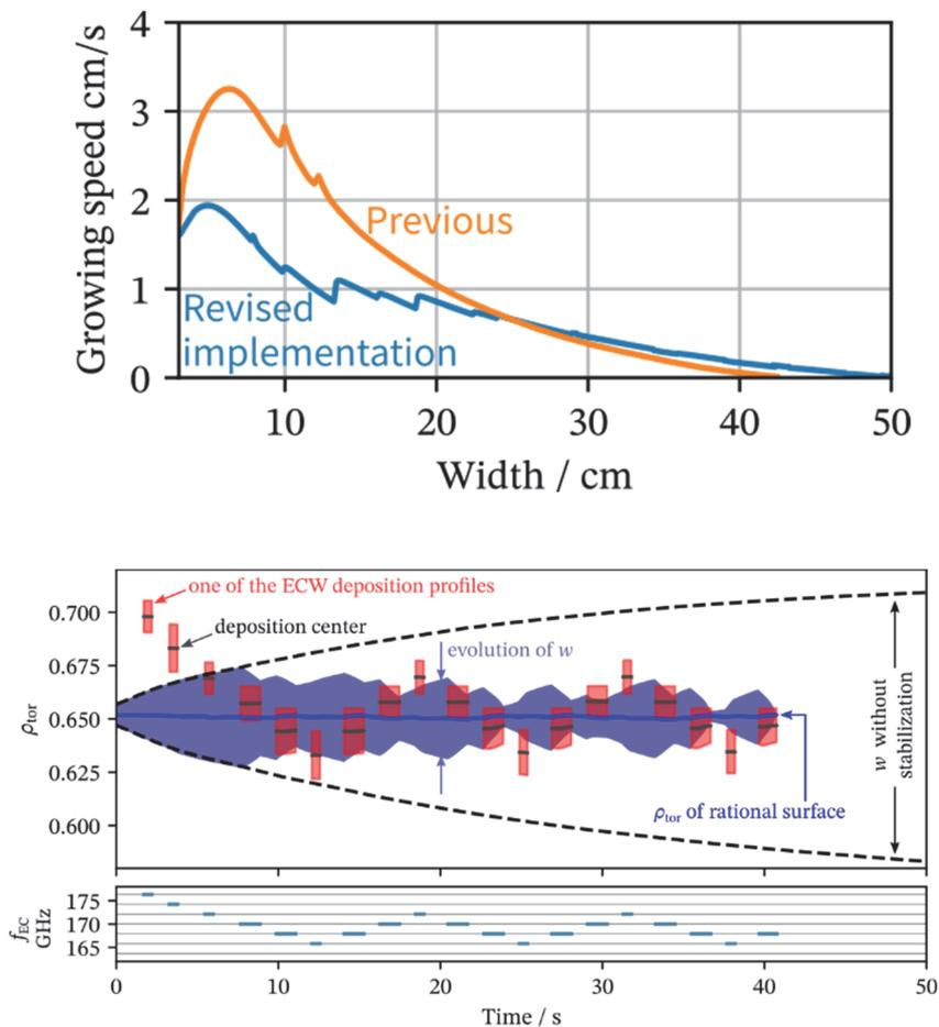
**Fig. 1.7.1:** Revised implementation of the modified Rutherford equation (top) and simulation of NTM control with tunable gyrotron frequency (bottom).
