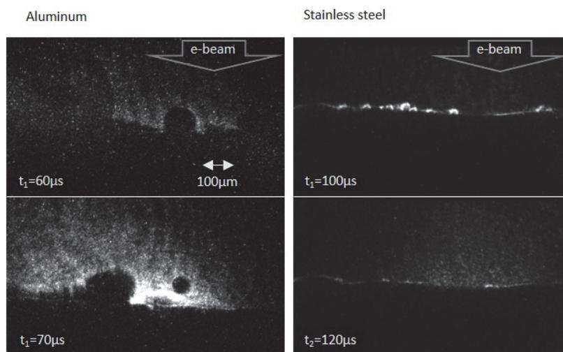
Fig. 3.1.1: 2D Schlieren imaging of droplets formation at the melt layers of aluminum and stainless steel.
