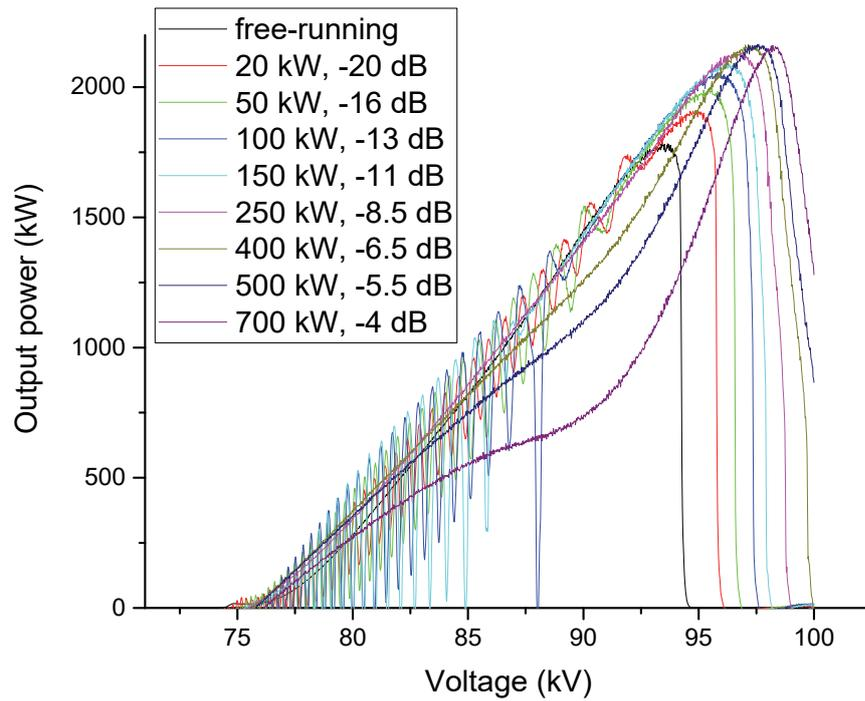
**Fig. 1.3.2:** Start-up scenarios for the TE<sub>34,19</sub> mode operating at the 2<sup>nd</sup> harmonic at 170 GHz for different levels of injected power.
