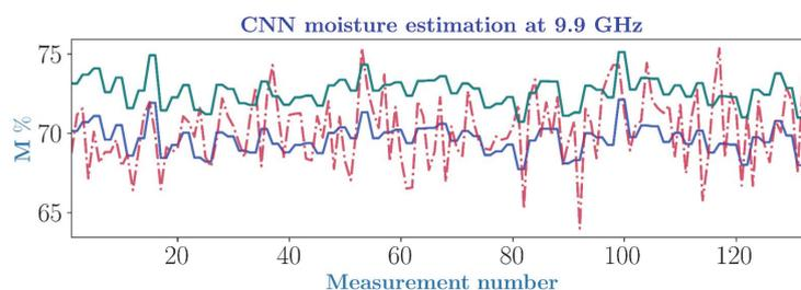
**Fig. 4.4.2:** Reconstructed image using CNN method, where blue lines are true moisture, green lines are true moisture uncertainty due to the weight, and red dash lines are reconstructed moisture value.
