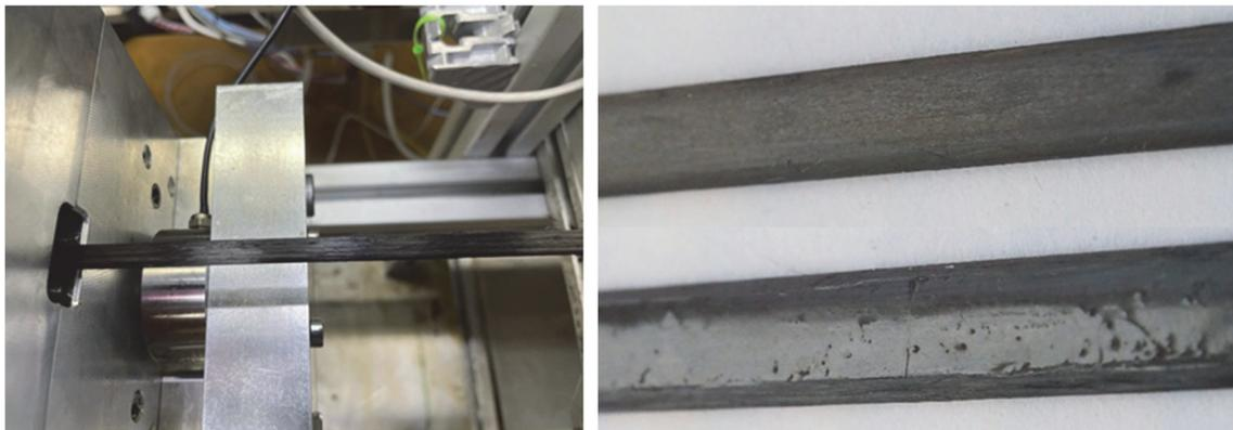
**Fig. 4.5.1:** Left: Fully cured profile exiting the microwave applicator; Right: Comparison of a profile of good quality with homogeneous cure (top) and a profile pultruded at insufficient microwave power (bottom) resulting in cured edges but wet resin on the flat surface of the profile.
