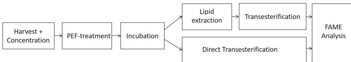
**Fig. 2.1.6:** Two possible routes to produce FAMES from microalgae. The direct transesterification process enables to bypass the lipid extraction, one of the most energy intensive step of downstream processing of microalgae.
