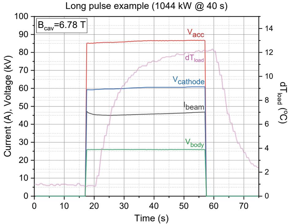
**Fig. 1.2.2:** Example of a 40 s pulse with 1044 kW peak power and 38 % efficiency (depressed collector operation).
