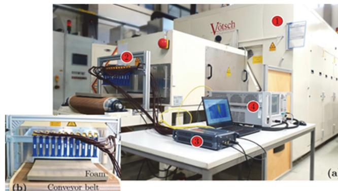
**Fig. 4.4.1:** (a) MWT system and its integration with the HEPHAISTOS (number Tag 1) is shown. The number Tags 2, 3, and 4 shows the MWT system, Solid state switch, and VNA respectively. (b) shows the enlarged view of the MWT sensor array of X-band open-ended waveguide antennas.
