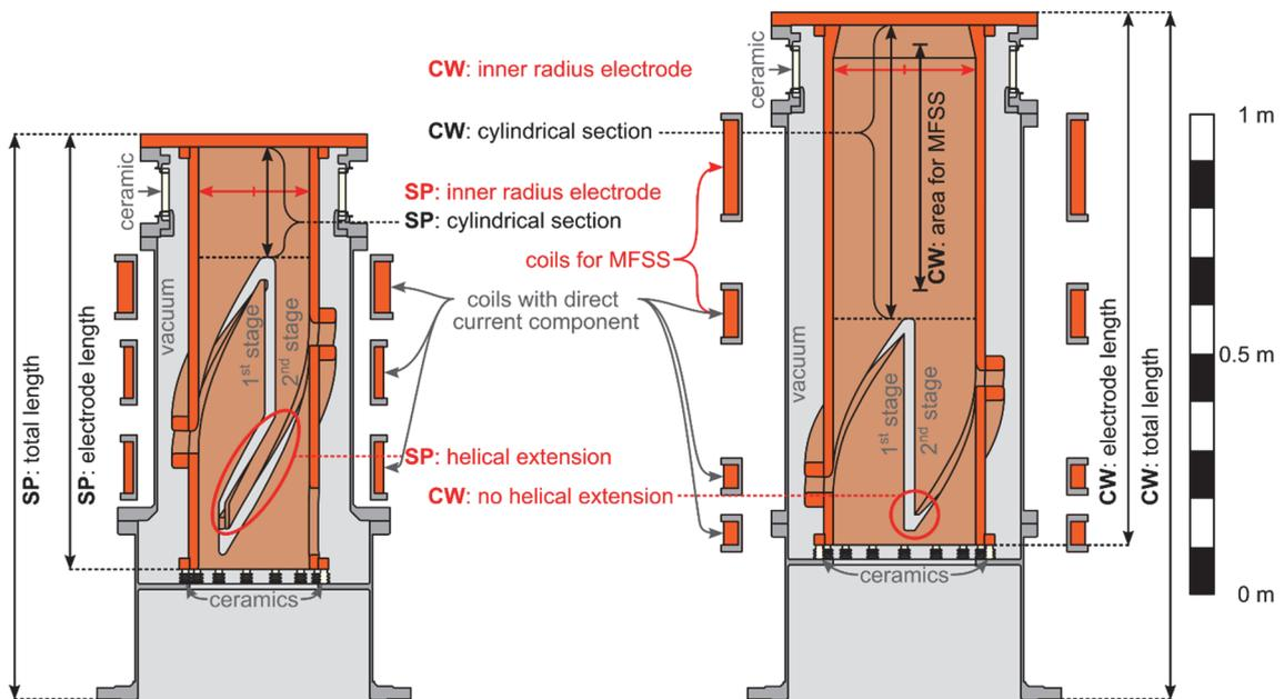
**Fig. 1.5.1:** Comparison between the short pulse MDC prototype (left) and the MDC design approach for continuous wave operation (right).
