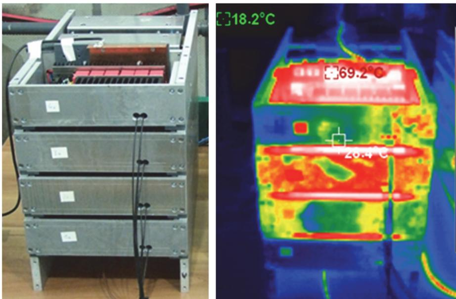
Fig. 2.2.3: Photo and thermographic image of one stack of four stages after 4.5 h of continuous operation at a total power of 9.7 kW, i.e. 1.2 kW per stage.
