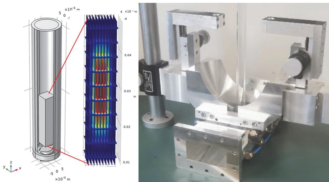
**Fig. 4.1.1:** CFD model of the surfaguide including heat source and helical gas flow (left) self-developed interferometer system mounted on the surfaguide plasma reactor (right).
