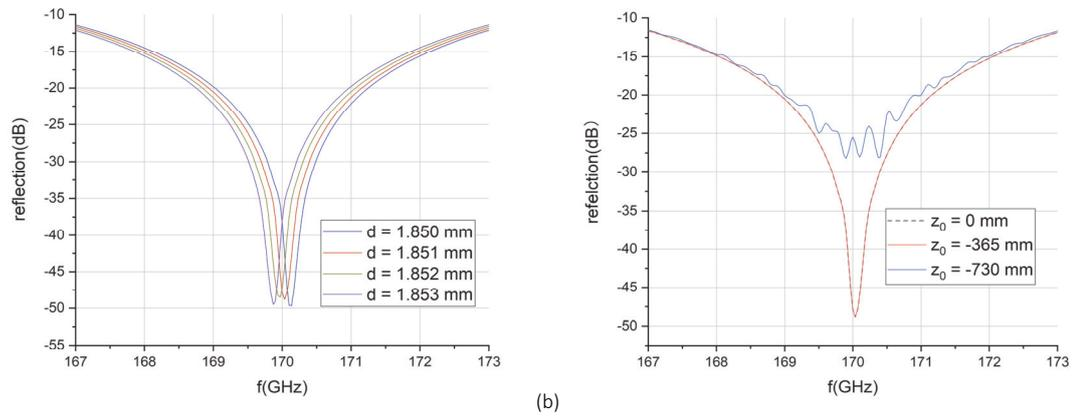
**Fig. 1.6.2:** Reflections of Gaussian beams on the diamond window: (a) without and (b) with gradient variation of wavefronts on the window disk.
