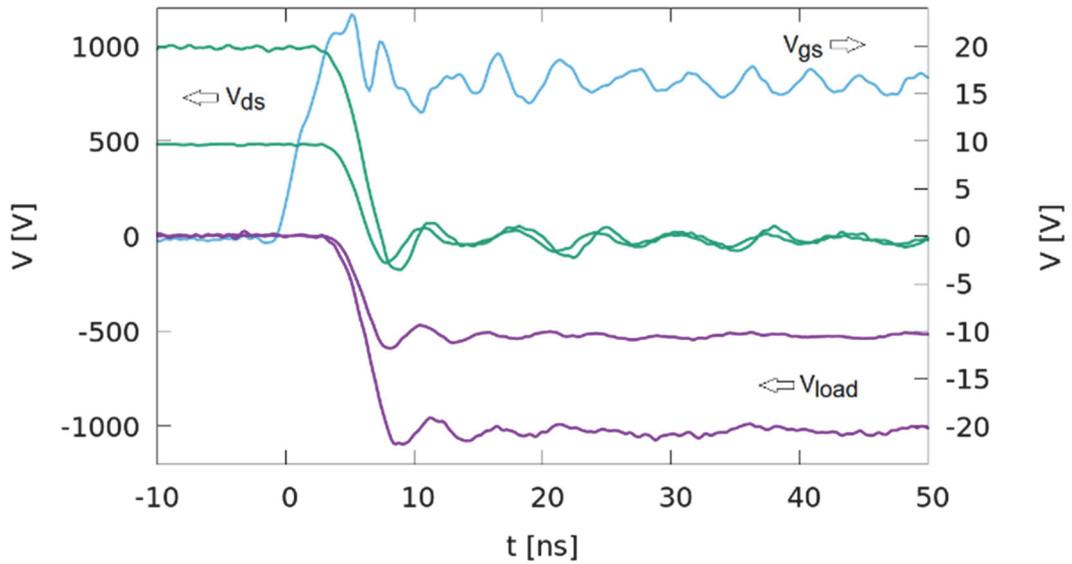
**Fig. 2.2.5:**  $V_{gs}$ ,  $V_{ds}$ , and  $V_{load}$  with gate boosting, charging voltage 500 V and 1000 V. (gate-boosting capacitance: 816 pF, driving voltage: 150 V).
