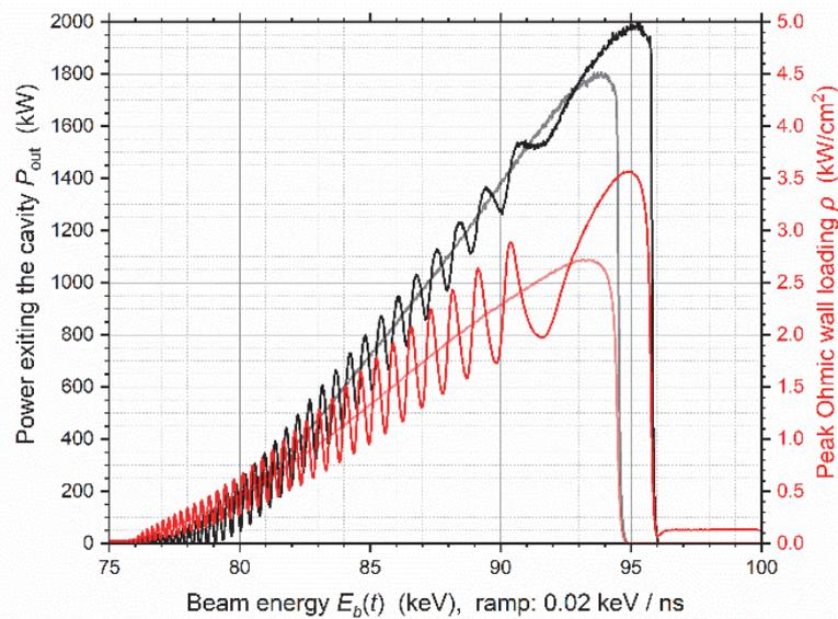
**Fig. 1.3.1:** Start-up scenario for the TE<sub>40,23</sub> mode operating at the 2<sup>nd</sup> harmonic at 204 GHz driven with 180 kW of injected power (black curve: output power, red curve: peak Ohmic wall loading). The results for the free running case are shown by the pale curves for comparison.
