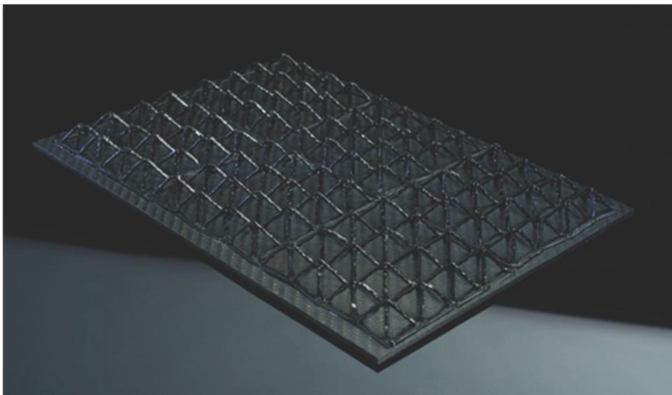
**Fig. 4.6.1:** 3D microwave printed lattice sandwich structure reinforced by continuous carbon fibers.
