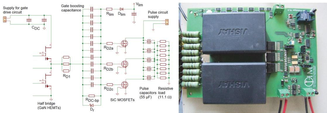
**Fig. 2.2.4:** Gate-boosting circuit featuring GaN-HEMTs in half-bridge configuration driving three paralleled SiC MOSFETs.
