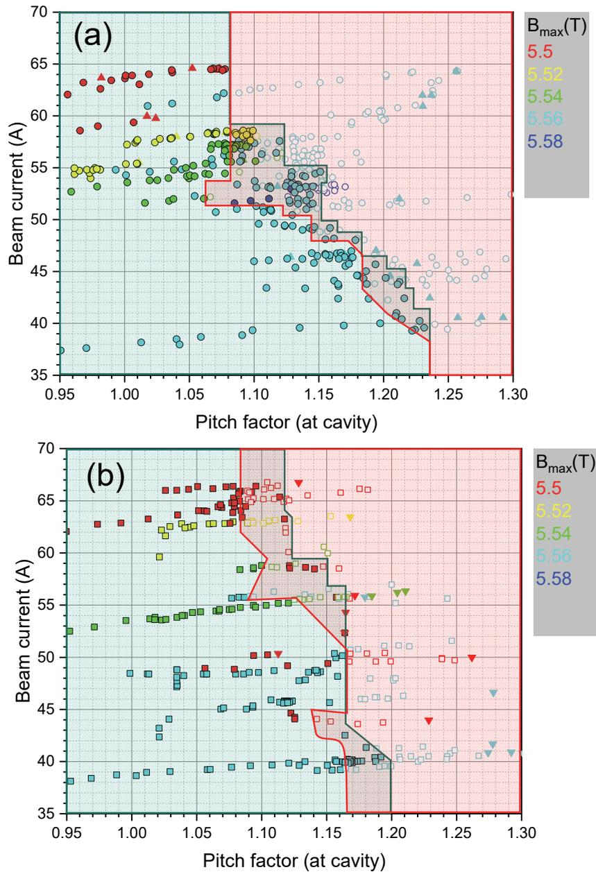
**Fig. 1.1.2:** Experimental pulses with the 1.5 MW short-pulse gyrotron placed on the current – electron velocity ratio (pitch factor  $\alpha$ ) operational space. The green container includes all parasitic-free pulses, whereas the red container includes all pulses with parasitics. (a) 1<sup>st</sup> campaign with baseline beam tunnel. (b) 2<sup>nd</sup> campaign with alternative beam tunnel.
