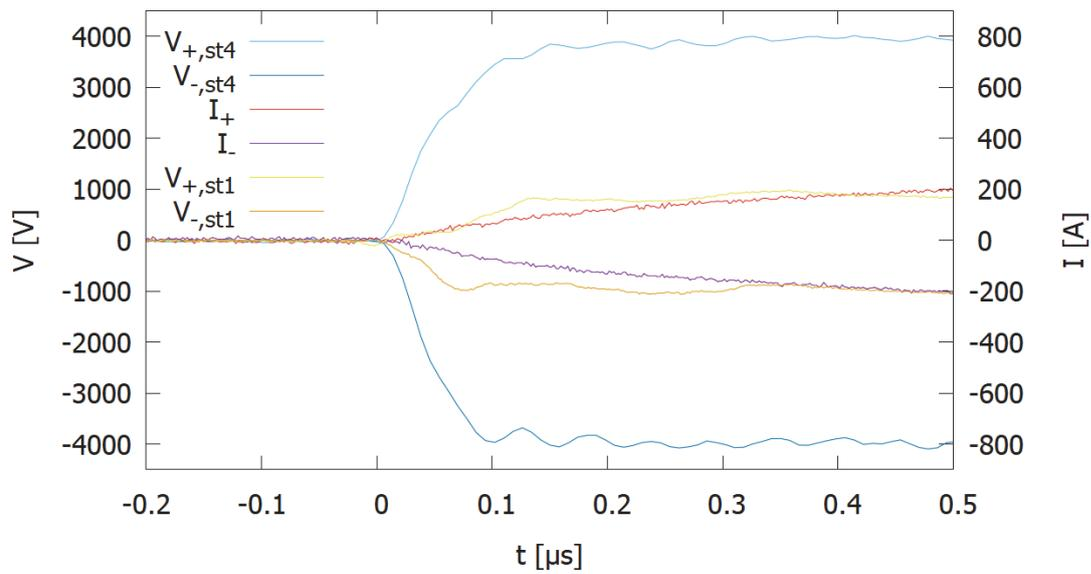
Fig. 2.2.2: Ground-symmetric operation of 8 stages at  $V_{stage} = 1$  kV and  $f_{rep} = 500$  Hz: Closing of the pulse switches under soft-switching conditions.
