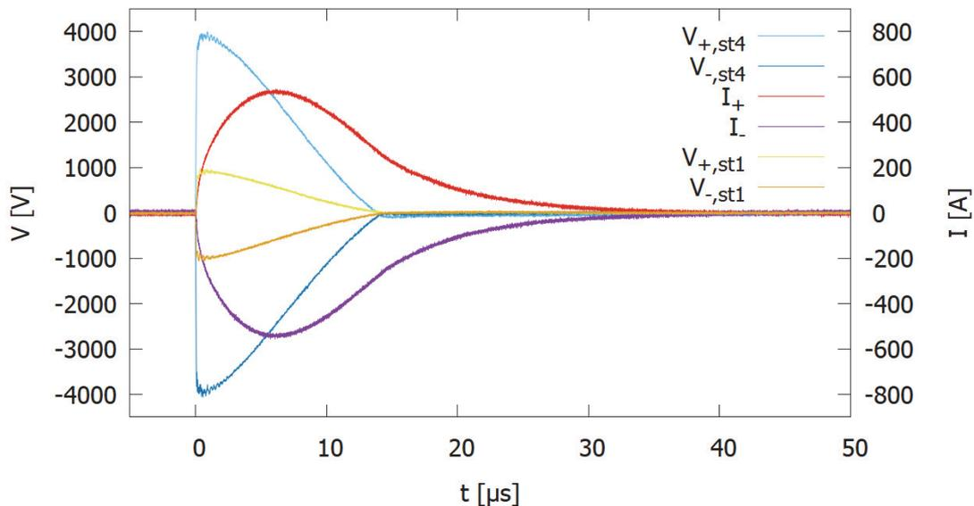
**Fig. 2.2.1:** Ground-symmetric operation of 8 stages at  $V_{stage} = 1$  kV and  $f_{rep} = 500$  Hz: Voltages and currents at the generator's positive and negative output terminal and at the outputs of both ground-side stages.
