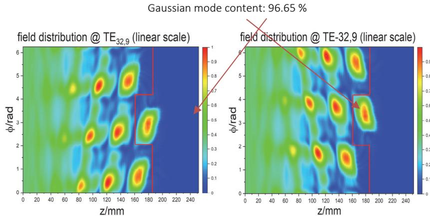
Fig. 1.6.1: Field distributions on the launcher wall and aperture @  $TE_{32,9}$  mode (left) and  $TE_{-32,9}$  mode (right).
