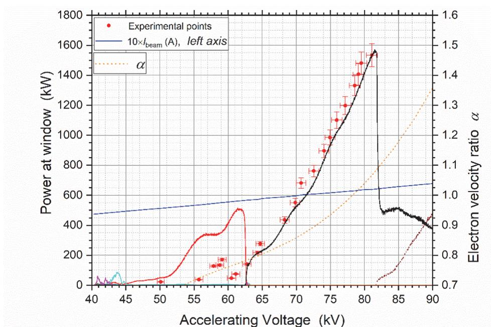
**Fig. 1.1.1:** Simulation/experiment comparison for the output power of the 1.5 MW short-pulse gyrotron. The black curve corresponds to the operating  $TE_{28,10}$  mode.
