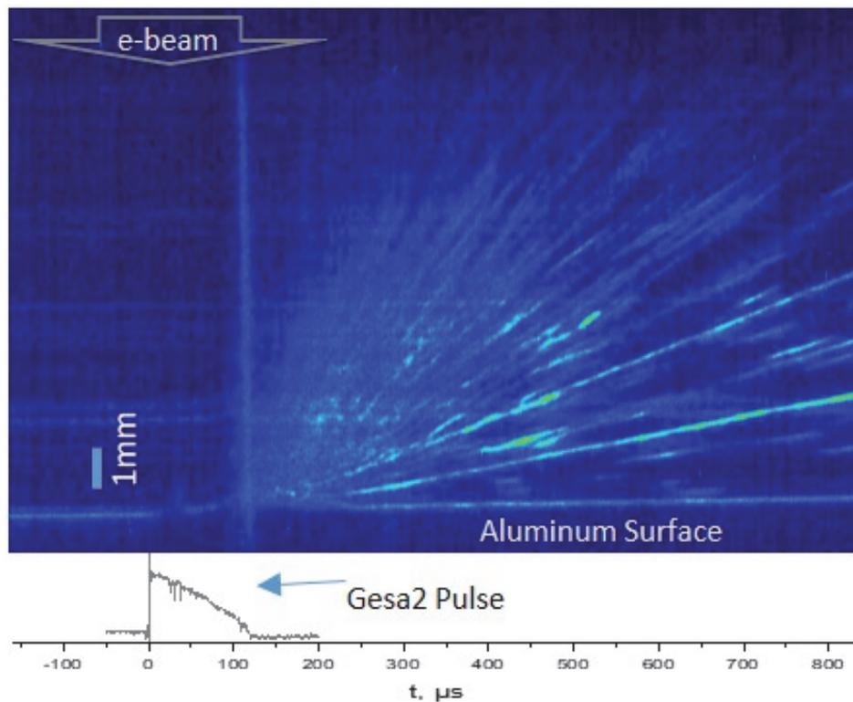
Fig. 3.1.2: 1D Schlieren imaging of droplets splashing from melt layer of aluminum, recorded with Streak-Camera.
