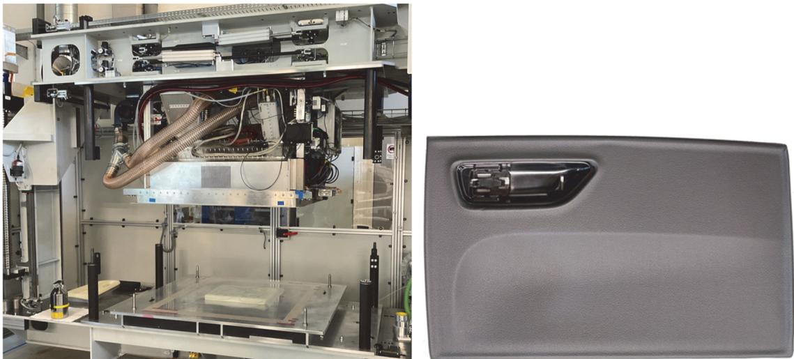
Fig. 4.2.1: e-KOMFORT microwave system (left); cover of a glove locker laminated with synthetic leather (right).
