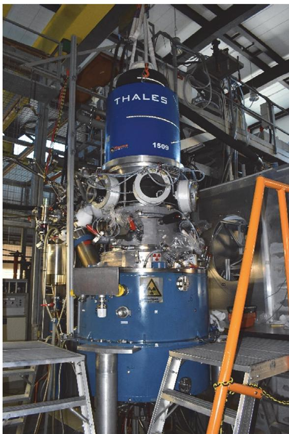
Fig. 1.2.1: EU ITER 170 GHz, 1 MW CW gyrotron installed in the test stand at IHM/KIT.
