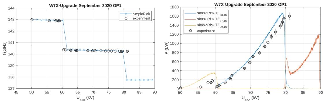
**Fig. 1.4.1:** Comparison of experimental and simulation results of the RF frequency (left) and power (right) at the gyrotron window for the pre-prototype 1.5-MW gyrotron for the upgrade of the electron cyclotron resonance heating system at the stellarator W7-X.
