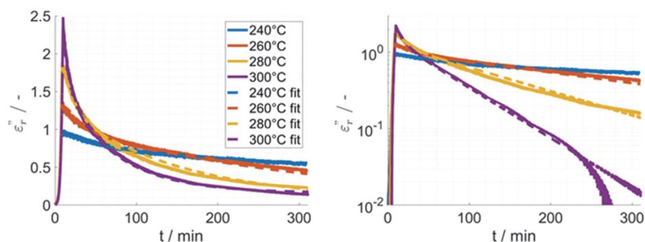
Fig. 4.3.1: Linear (left) and logarithmic (right) graphical presentation of the measured dielectric loss and the fitted curves.
