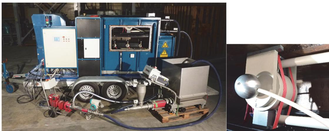
**Fig. 2.1.2:** New treatment chamber integrated into the PEF Demo-facility, right, and setup for the fatigue test at the technician at KIT-IHM, left.
