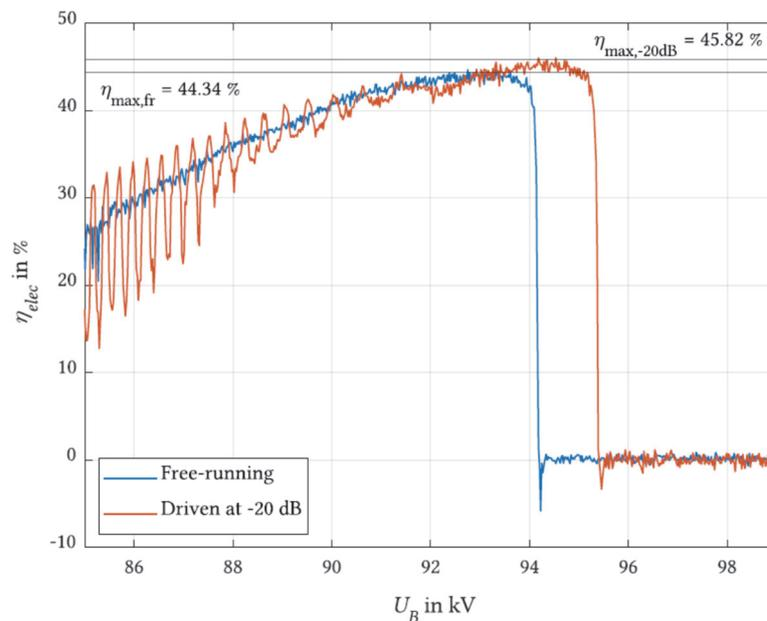
**Fig. 1.9.1:** Electronic efficiency versus beam voltage (increasing at a rate of  $\sim 0.03$  kV/ns) for the 170 GHz 2 MW coaxial gyrotron. In the driven case, a 30 kW external signal at 169.972 GHz is used. The oscillations appearing below 92 kV in the driven case reflect the non-locked regime. From 92 kV onwards, the frequency of the operating mode is locked to the injected frequency.
