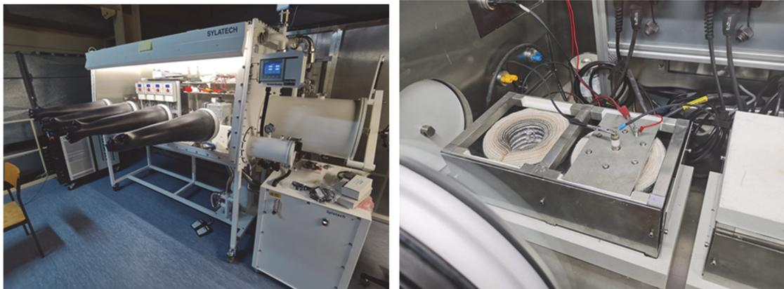
**Fig. 2.3.3:** Glove box with the test facility and a battery under testing.
