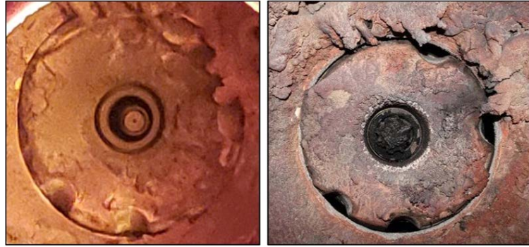
Figure 14: Burner during and after experiments
