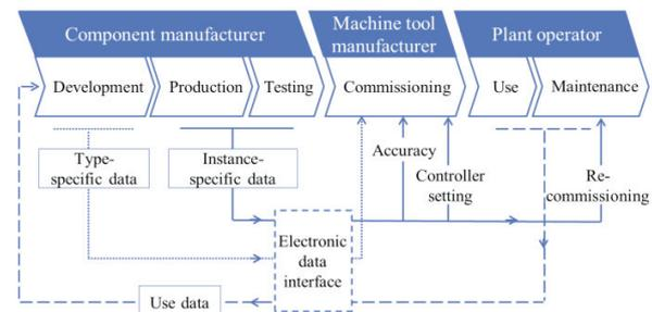
Fig. 3: Data flows over the life cycle of a networked machine component
