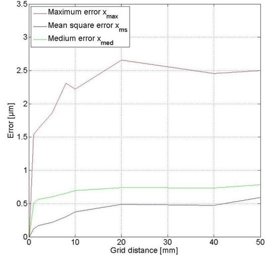
Fig. 7: Error relative to grid distance
