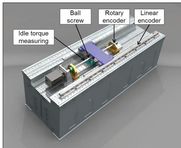
Fig. 9: CAD model of test bench
