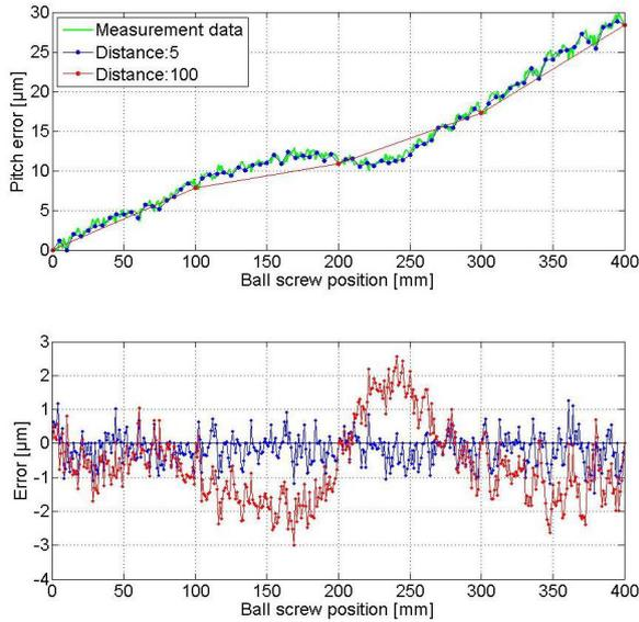
Fig. 6: Pitch error and relative error
