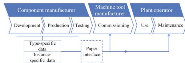
Fig. 1: Life cycle of a machine component
