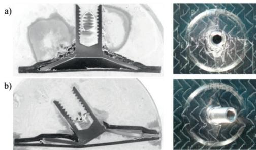
Fig. 5. Polished cut images and pictures of the failed specimens of the a) tensile tests and b) bending tests
