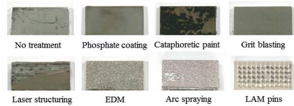
Fig. 11. Fracture surfaces of the metal parts of the specimens
