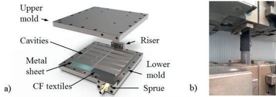
Fig. 9. a) RTM mould for the manufacturing of the specimens, b) used test device with a single lap joint specimen
