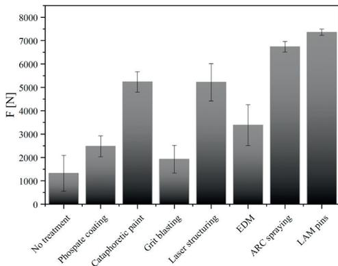
Fig. 10. Tensile load bearing capacity of the single lap joint specimens with different surface treatments/coatings of the metal sheets
