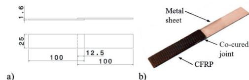
Fig. 8. a) Dimensions of the specimens b) exemplary picture of a specimen
