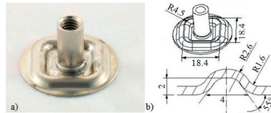
Fig. 6. a) Tested insert with a bead pattern b) Dimensions of the used bead pattern
