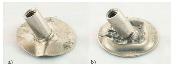
Fig. 7. Deformation of an insert without (a) and with a bead pattern (b)
