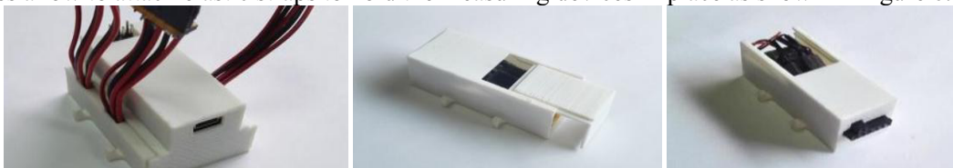
Figure 6. Housings for mainboard (left), sensors (center) and batteries and Bluetooth module (right)
