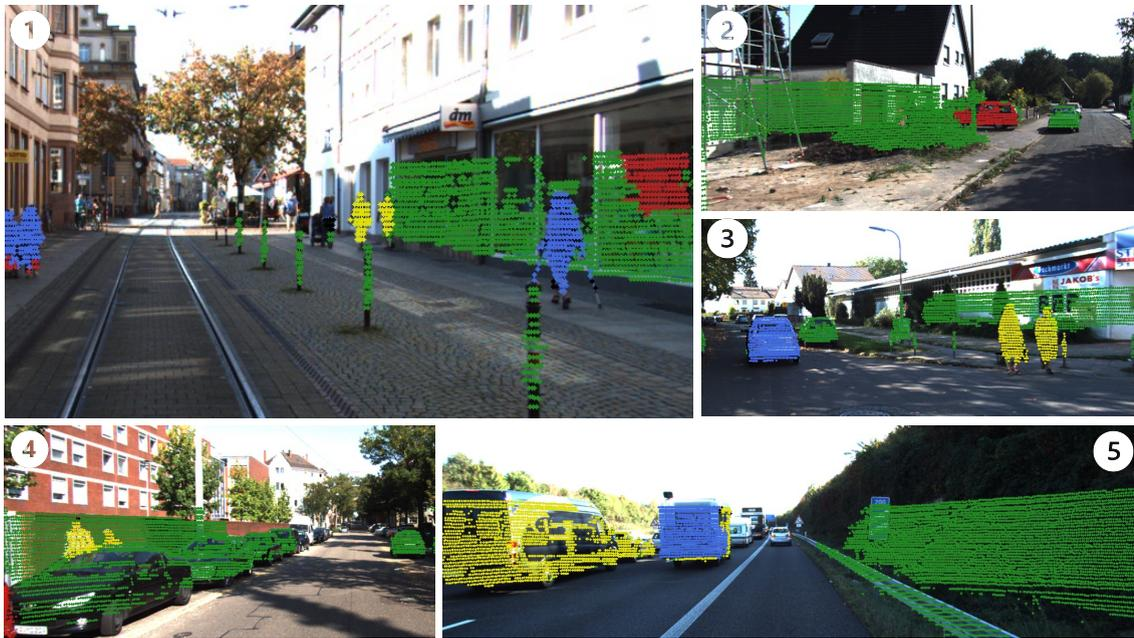
Figure 4.6: Examples of anomalies where the SV part of my method correctly classified. The anomalies are shown in yellow and red.
