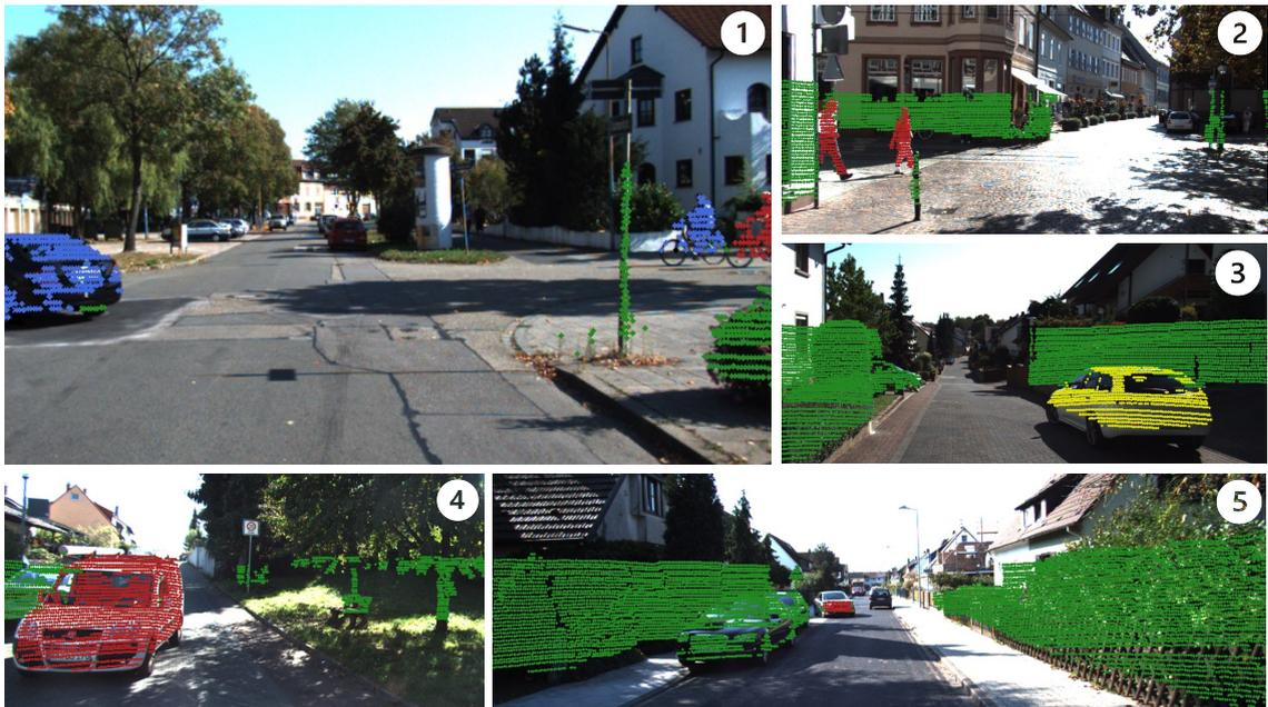
Figure 4.5: Examples of anomalies where the SSV part of my method correctly classified. The anomalies are shown in red and yellow.
