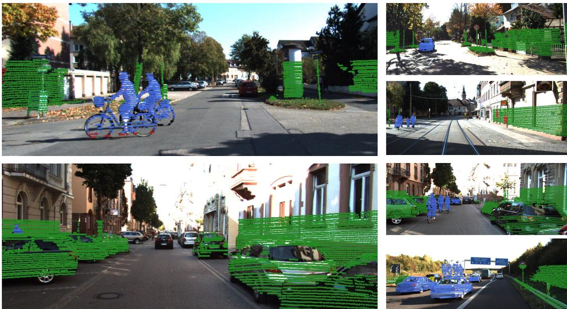
Figure 4.3: Examples where the SV and SSV parts are correctly consistent. Dynamic points are classified as dynamic (blue) and static points as static (green) by both parts.
