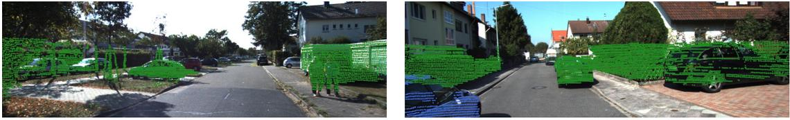
Figure 4.4: These two images show points of objects that were misclassified by both parts of my method. The left image shows two pedestrians classified as static, and the right image shows a parked car classified as dynamic.
