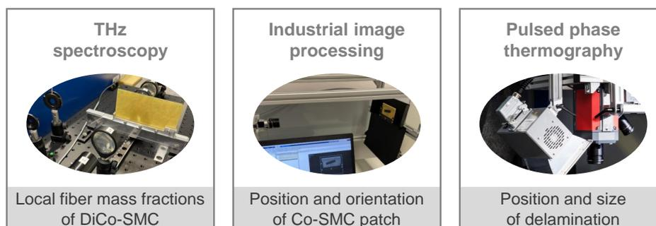
*Figure 5.1: Proposed measurement technologies and respective measurands for CoDiCo-SMC*
