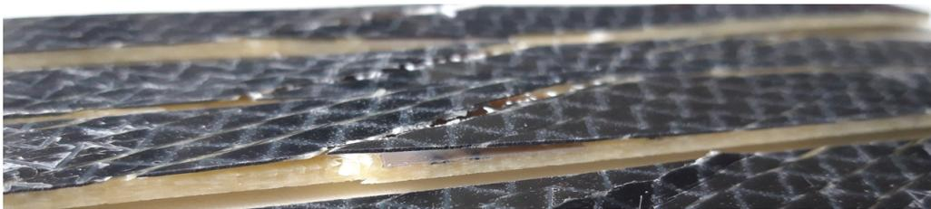
(b) Inter fiber fracture of Co-SMC (41.20.T20)
