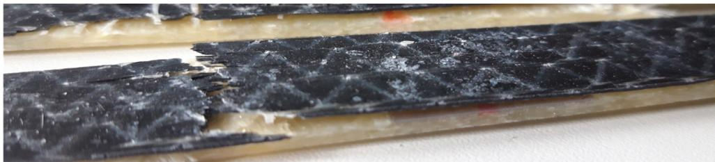
(a) Fiber fracture of Co-SMC (41.0.T20)
