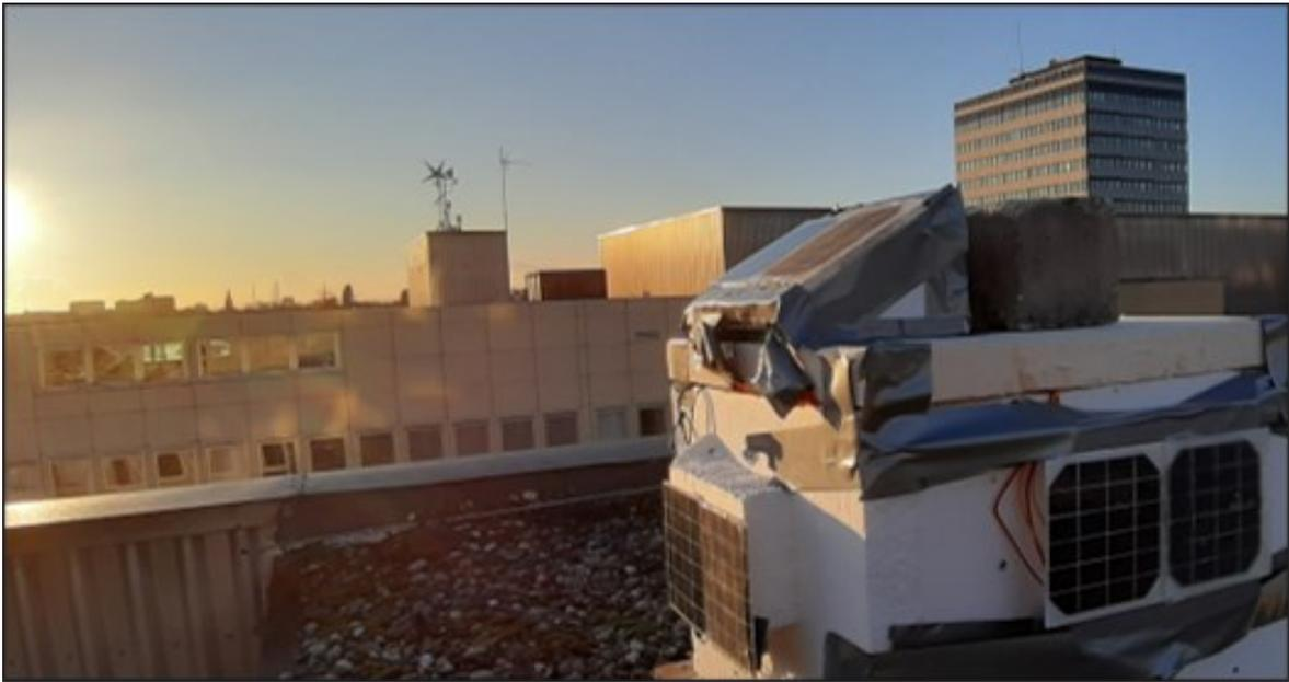
**Fig. 9.1:** Photograph of the setup developed for outdoor performance monitoring of PV modules with and without rose petal textured PMMA light-harvesting cover layers. The depicted modules were installed under  $30^\circ$  and  $90^\circ$  tilt towards the south, as well as under  $90^\circ$  tilt towards the east.
