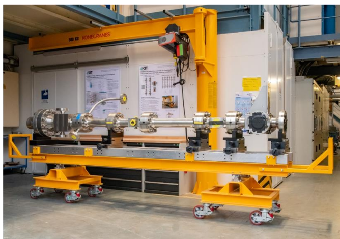
Figure 10 Pressure hull of the test section including high-pressure windows (l) and fragment shields (r)
