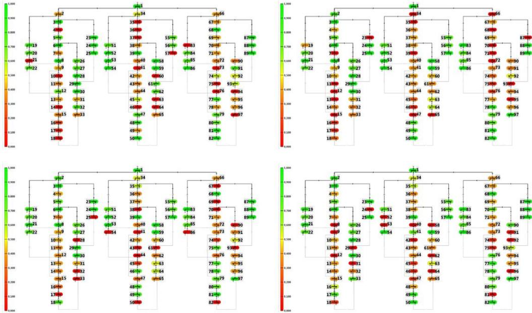
Figure 2 Heat map of the relative power supplies: in contrast to the rolling blackout of Fig. 3 continuous power flows are realised in an urban resilient, fair and efficient way over four time steps (red colour indicates induced blackout) [16]
