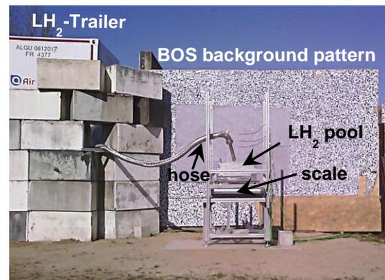
Figure 1: POOL-facility set-up for the unignited and ignited LH<sub>2</sub> pool experiments of the PRESLHY project.
