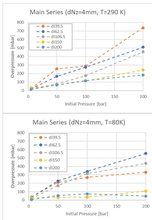
Figure 9. Maximum measured overpressures in experiments at ambient (top) and cryogenic temperature (bottom) of the discharged gases.
