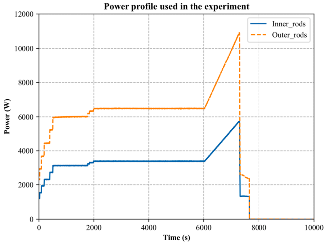
Fig. 9. Established power profile for inner heated rods and outer heated rods.
