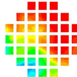
FLUENT: 3D Thermal Hydraulics model of downcomer and lower plenum
