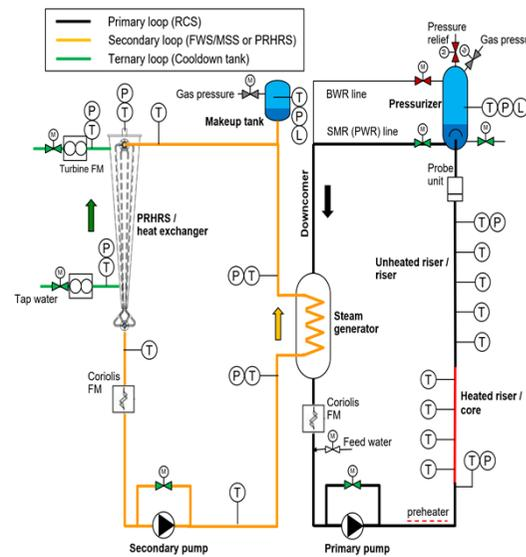
HWAT experimental setup for transient tests under natural circulation
