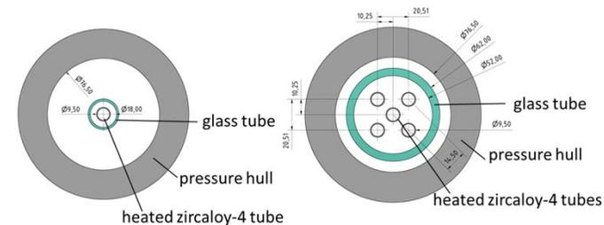
**Cross-sectional view of the two planned test arrangements**
