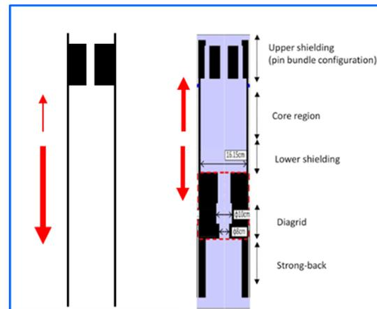
Transfer Tube: simplified layout (left) used in simulations
