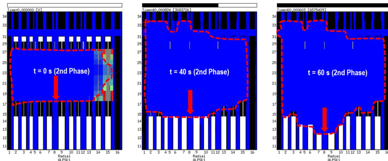
The poorly cooled core slowly settles down: plugs are melted to form again deeper down. Once the LAB and LGP etc. are destroyed, the core inventory is relocated to the CC.
