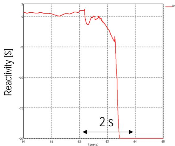
Discharge through 7 TT (out of 31) leads to deep subcriticality in less than 2 s.
