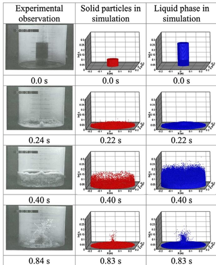
Sloshing experiment (KIT) and numerical simulations
