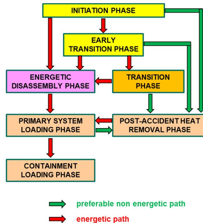
Fig. Phases of a severe accident
