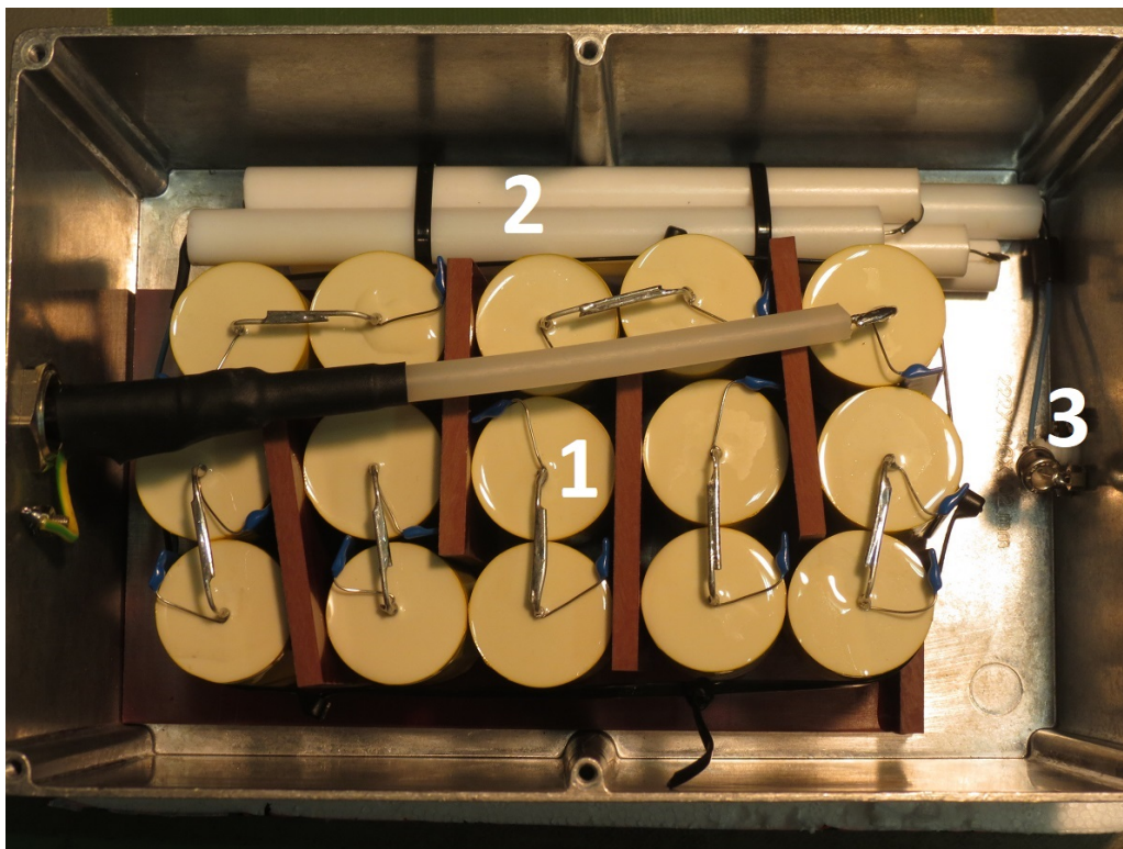
Figure 8. Picture showing the interior of the ripple pick-up probe. The device consists of 15 series-connected 150 nF / 3 kV foil capacitors with balancing resistors (1), a surge protection resistor chain (2), and a gas discharge surge arrester (3). All components are embedded in silicone potting that has not been applied in this photo yet. The width of the enclosure is about 21 cm.
